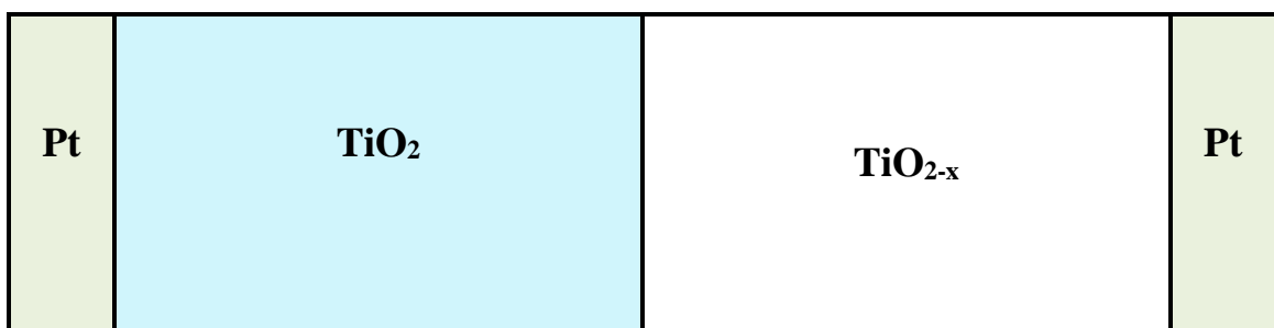
Figure 3.2: Memristor device structure presented by S. Williams and his research group at HP laboratories [16].
