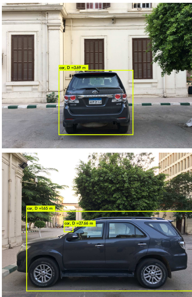
Fig. 1. The distance at 3.69m from back view and 1.65 from side view “side view problem”
