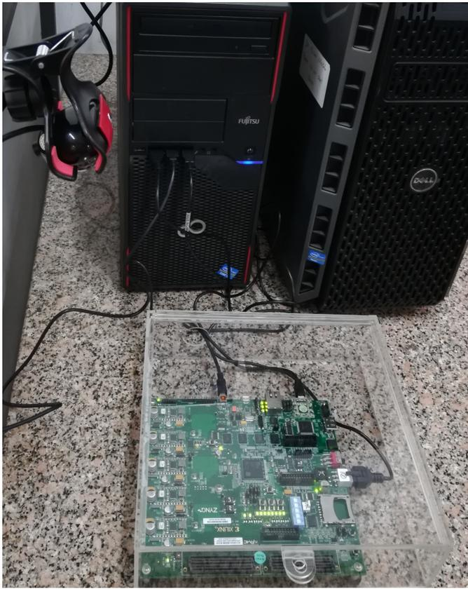
Fig. 4. ZC702 Evaluation board connected to a server with webcam mounted on top of it.
