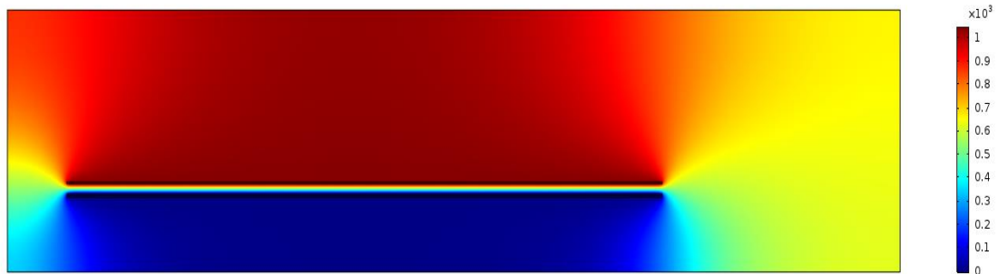
Figure 3.2 Calculated potential distributions at the attached electrode contact mode conductor-to-dielectric when x=1360\mu\text{m}
