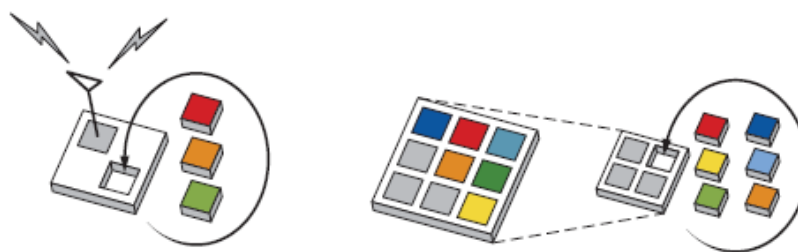
Figure 4.6: Modifying Functionality and Reducing Size using Partial Reconfiguration [13]
