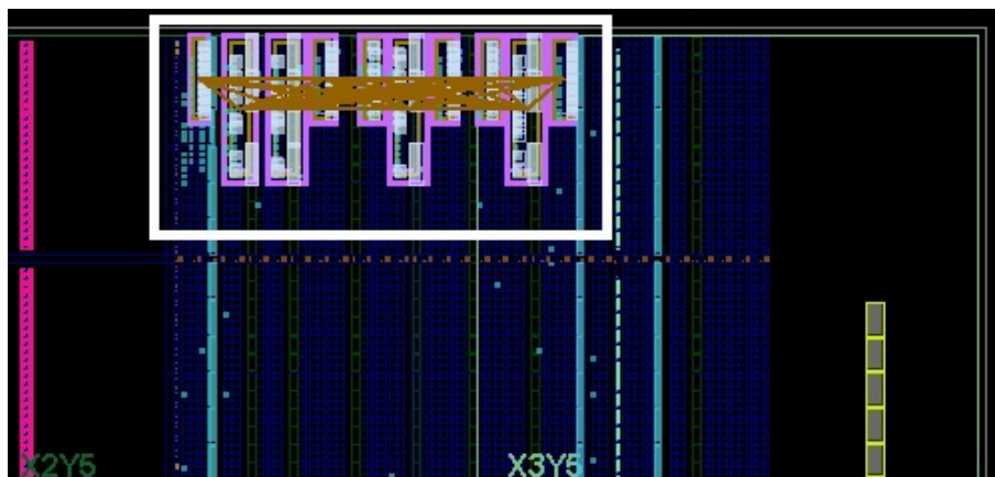
Figure 14. Floorplanning and static routing (reconfigurable area) of the physical neurons in case of the SVHN dataset.
