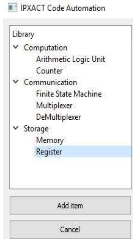
Fig. 3 Main building blocks window. The user adds from this library the blocks he needs in order to design his system.
