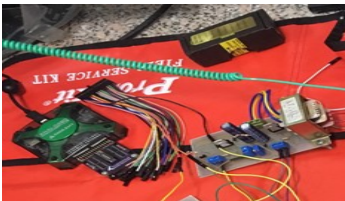
Fig. 4.2 Memristor programming using Known Kit along with analog discovery board.
