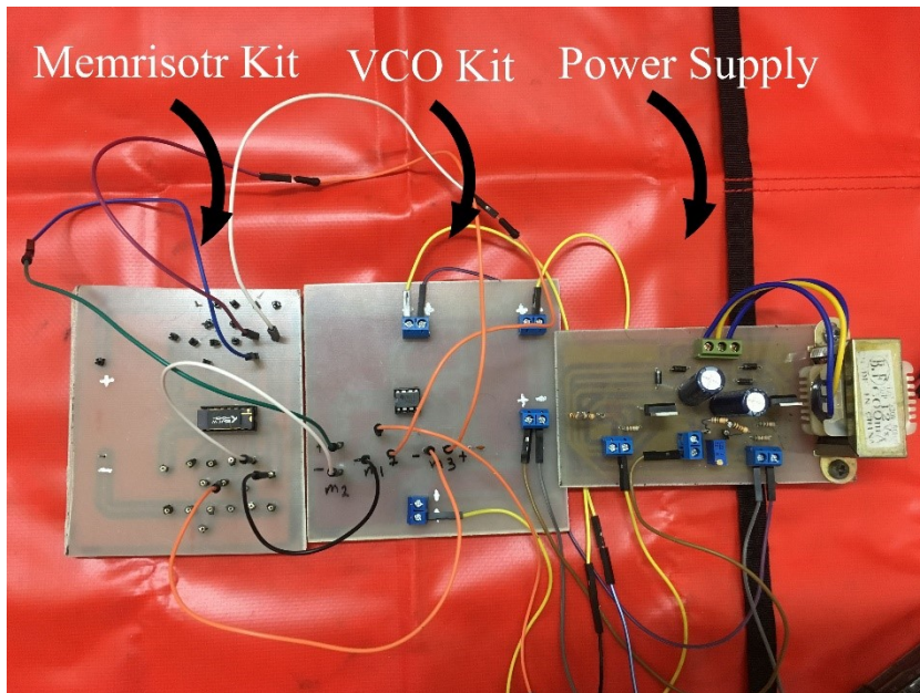
Fig. 4.7 The complete printed circuit boards (PCBs) arrangement for implementing the memristor-based VCO prototype circuit.
