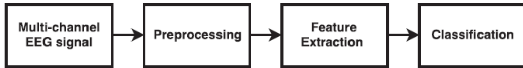
Figure 2.4: Automatic seizure detection system
