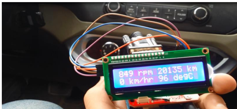
Figure 67 - Displaying the values of engine RPM, distance travelled, vehicle speed, and engine coolant temperature of a stable car
