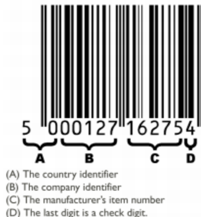
Figure 2.2: the structure of a barcode in EAN-13
