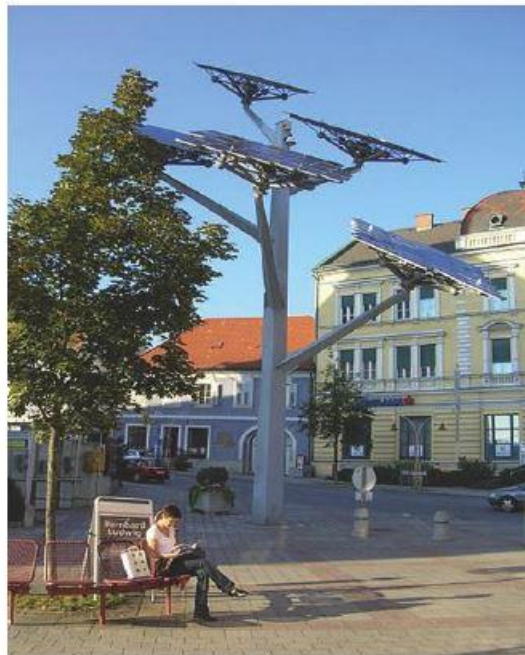
Figure 34 Example of solar tree in Austria (Gleisdorf) [2]
