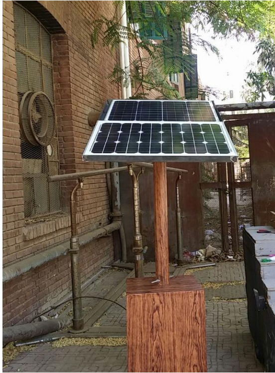
Figure 33 Solar Tree Prototype
