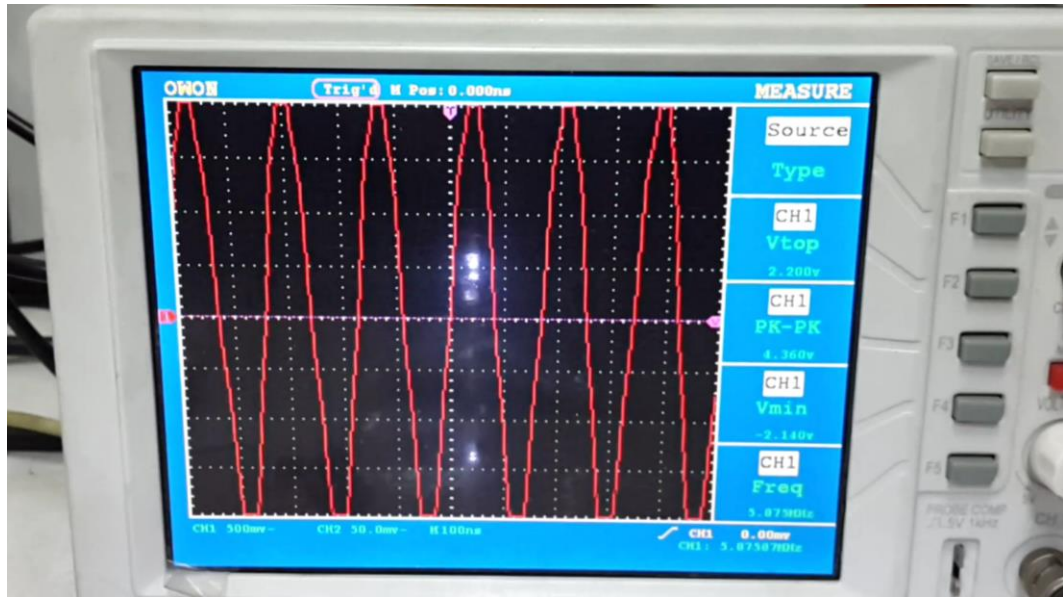
Figure 33-Sensor after one amplifier at frequency 5MHZ with 4.5v pk-pk
