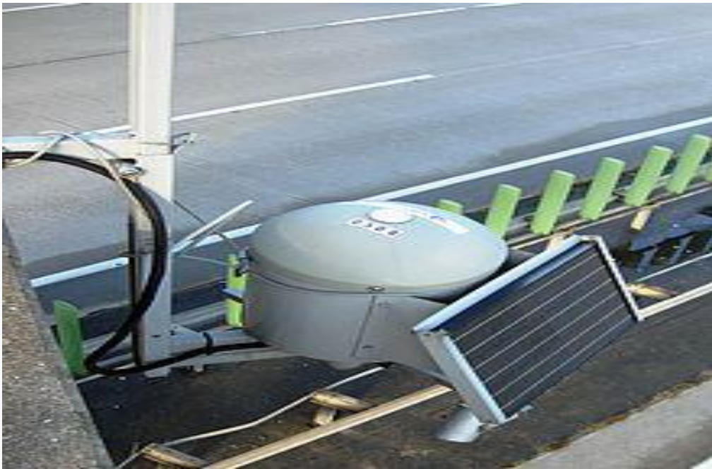
Figure 3.3 Traffic congestion detectors in Germany.
