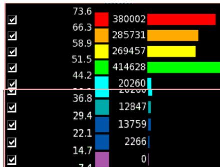
From the above map the maximum IR drop is 73.6 mV which is 7.75% of the used power supply value which is 950 mV and this drop is acceptable since it's lower than 10% limit recommended by Synopsys.
