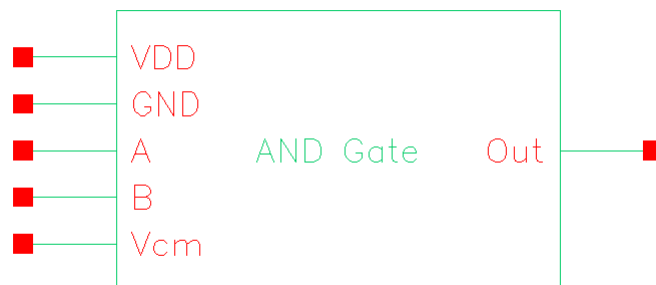
Figure 5.33: Symbol of the AND gate
