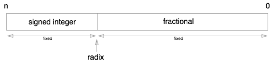
Figure 21: Fixed-Point representation of numbers
