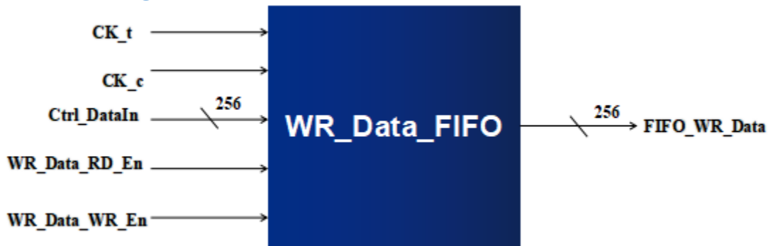
Figure 10: Block Diagram of Write_Data_FIFO
