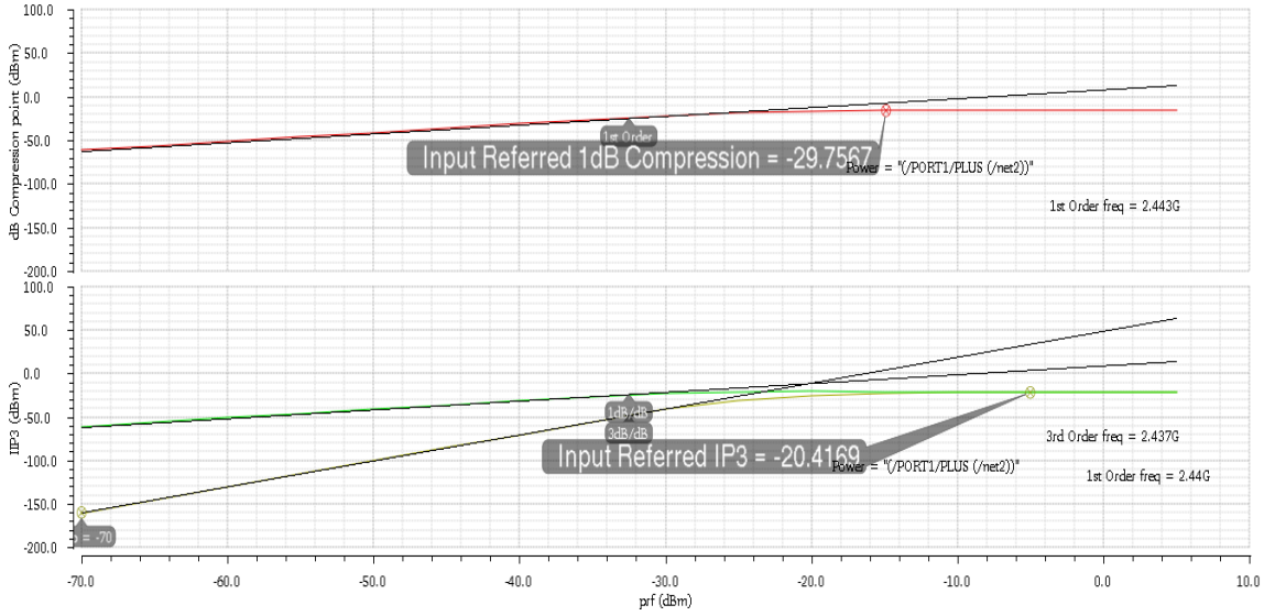
(a) First mode linearity factors of the whole LNA architecture
