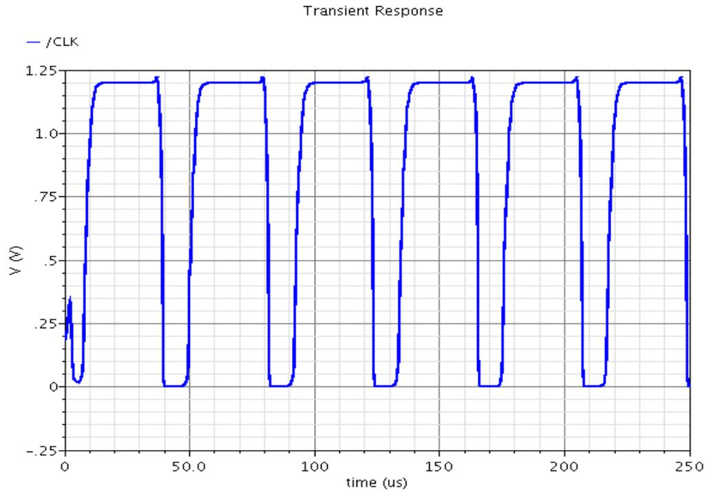
**Figure 3-25: Post-layout simulations of the oscillator**
