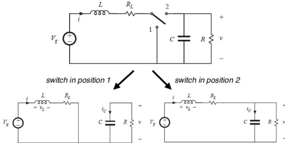
**Figure 2-9 Model of the DC resistance**
