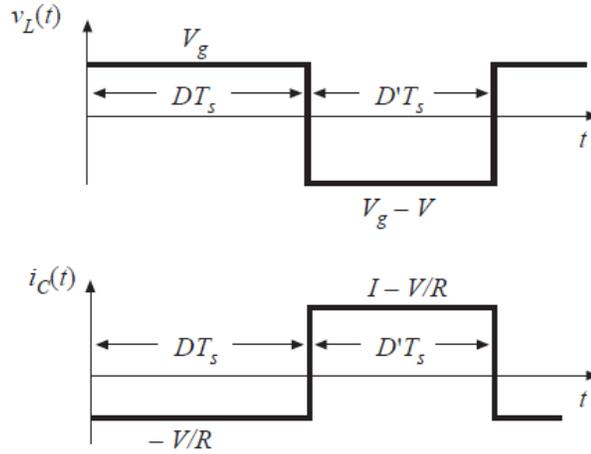
**Figure 2-7 combining the two modes with the duty cycle action**
