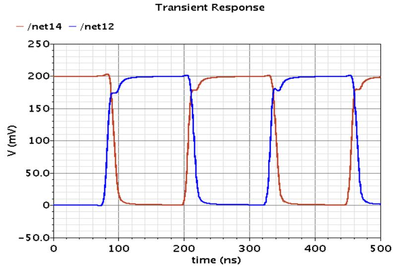
Figure 5-11 post Layout simulation of clock driving charge pump
