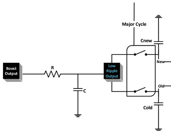
**Figure 2-14 Switching circuitry**
