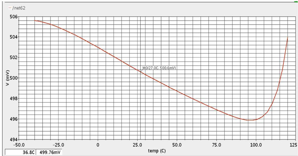
**Figure 4-13 output voltage variations at SS corner after using a trimming circuit**
