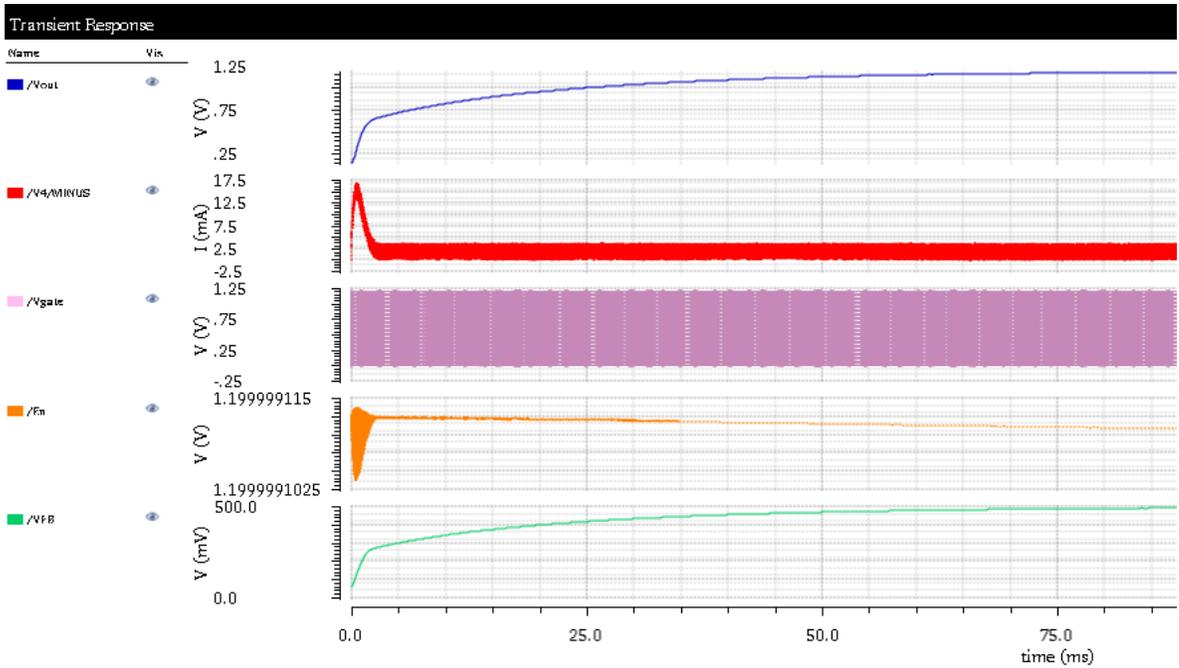
**Figure 3-19: Simulation results of the output regulation stage at  $V_{in} = 200$  mV**
