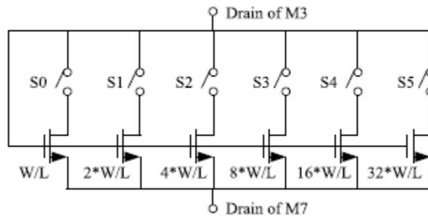
**Figure 4-12 using M11 as a trimming circuit**
