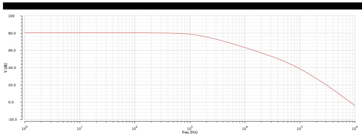
**Figure 3-17: AC simulation of the Feedback Comparator**
