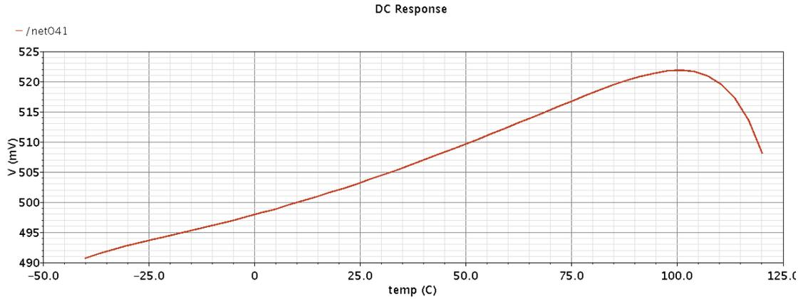
**Figure 4-19 Layout simulation of Band gap core**
