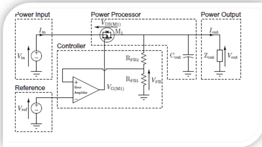
**Figure 3-4: Block diagram of a typical LDO using a PMOS**
