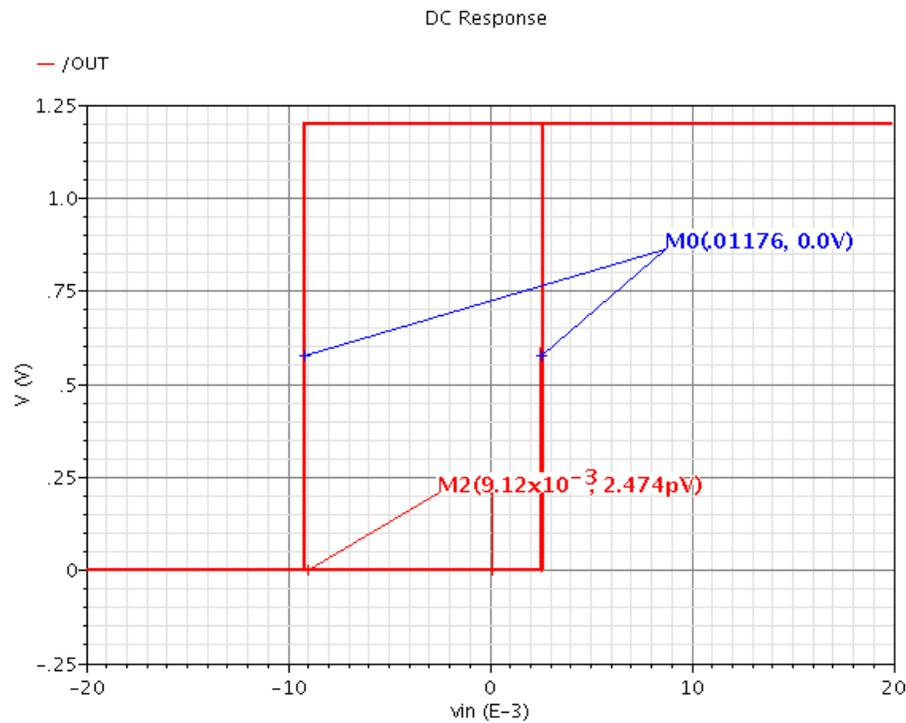
**Figure 2-36 Post-Layout simulations for hysteresis window**
