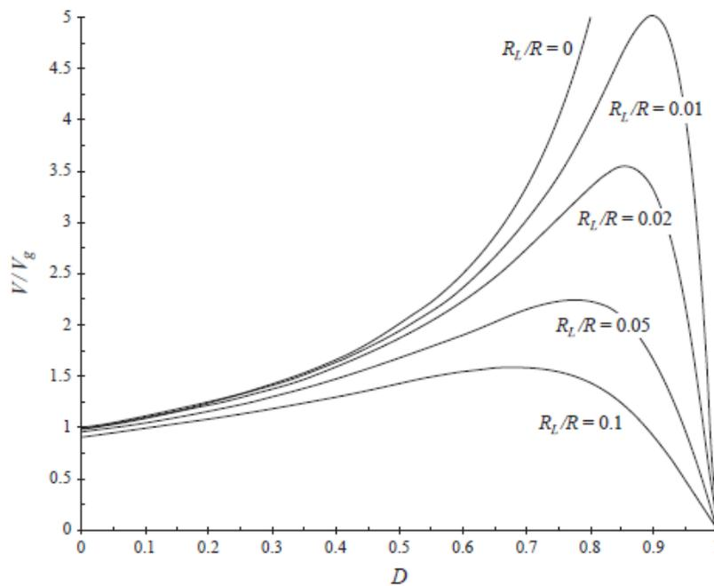
**Figure 2-10 Stability curves vs the dc resistance relativity values**
