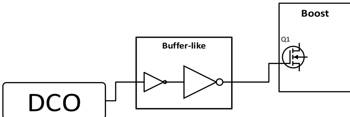
Figure 2-23 Gate driver between boost converter and DCO
