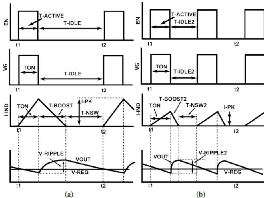
**Figure 3-11: Conceptual waveform of the PFM mode converter. (a) Typical single pulse operation. (b) Single pulse operation with decreased input voltage as compared to situation shown in (a).**
