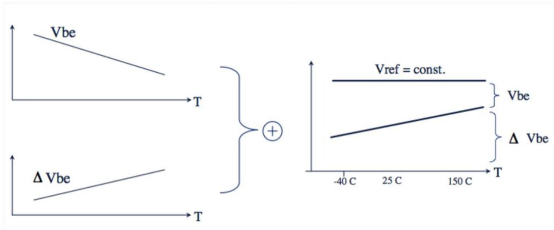
**Figure 4-1 Temperature compensation using BJTS**
