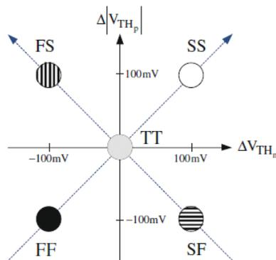
**Figure 2-27 corner simulations vs change in threshold voltage**
