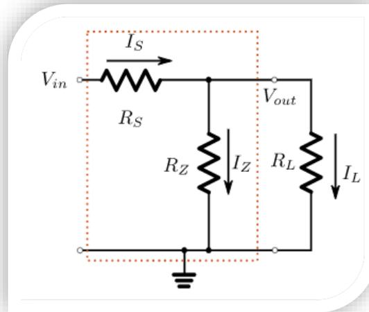
**Figure 3-2: Linear regulator core**
