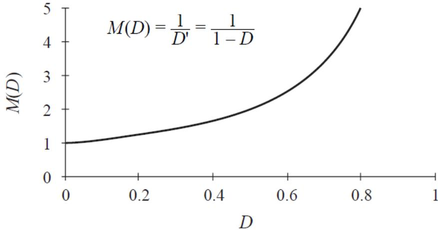
**Figure 2-8 action of duty cycle vs the conversion ratio value**
