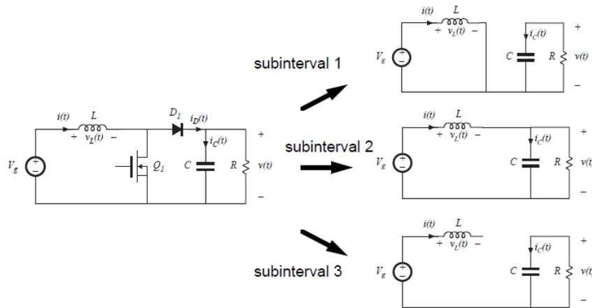
**Figure 2-11 Modes of operation of DCM boost converter**
