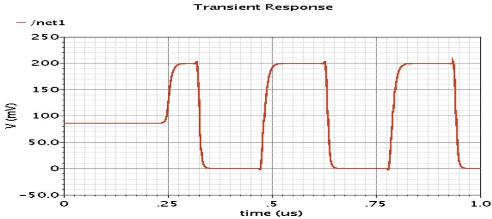
**Figure 5-5 post Layout simulation of oscillator**
