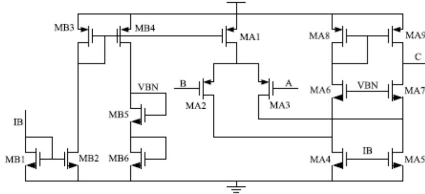
**Figure 4-3 Schematic of OPA used in the proposed sub-BGR**
