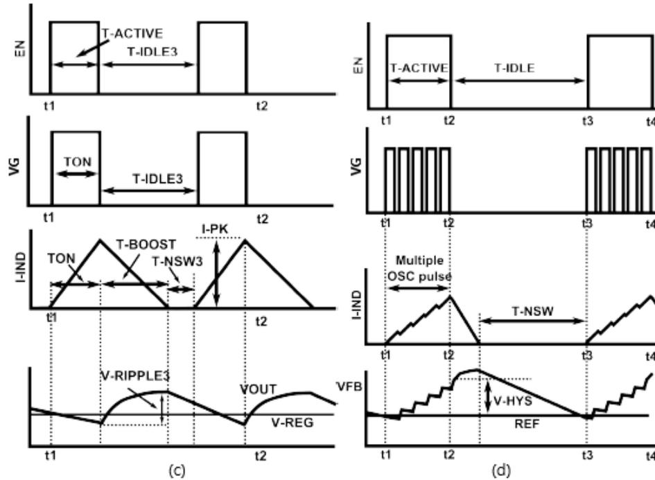
**Figure 3-12: Multi pulse operation (a) Single pulse operation with increased load as compared to the condition shown in Fig. 3-11a. (b) Multi pulse operation, when the converters idle time is exhausted due to increased load or conversion ratio or for both**
