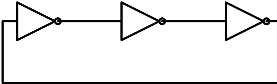
Figure 2-18 3 stages ring oscillator
