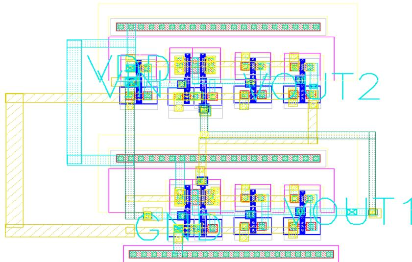
**Figure 5-7 Layout of non-overlapping clock generator**
