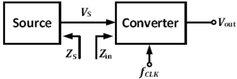
**Figure 2-3 Matching the source and load impedance**
