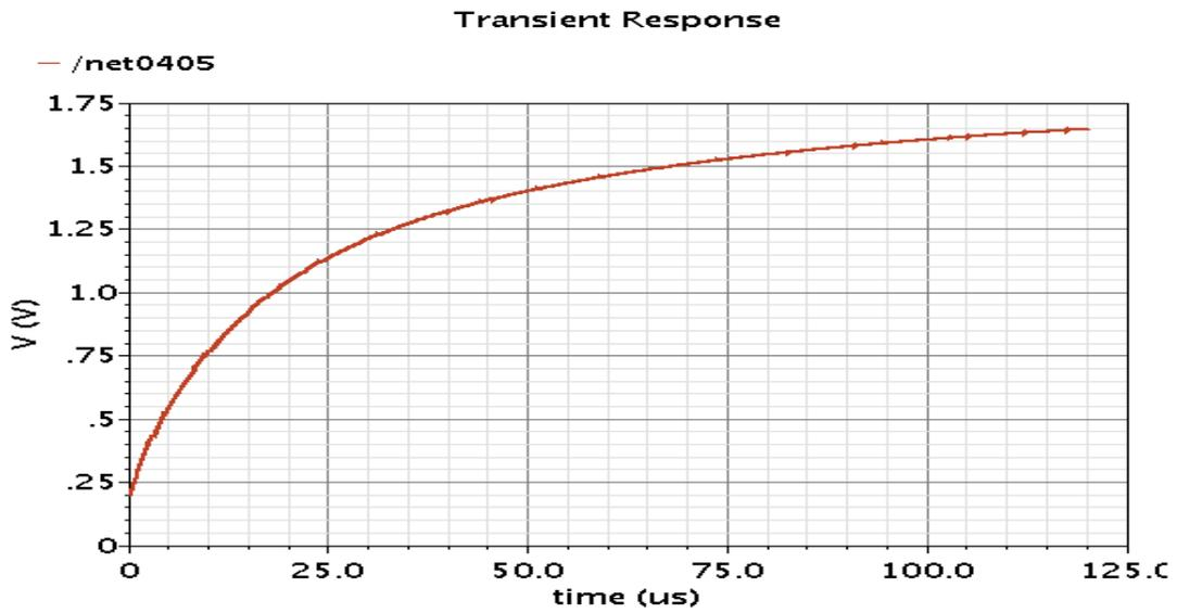
Figure 5-17 cold start output @ vin=0.2v
