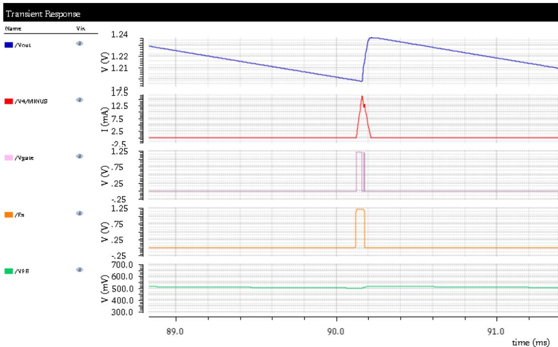
**Figure 3-24: Magnifying the simulation results of the output regulation stage at  $V_{in} = 900$  mV**
