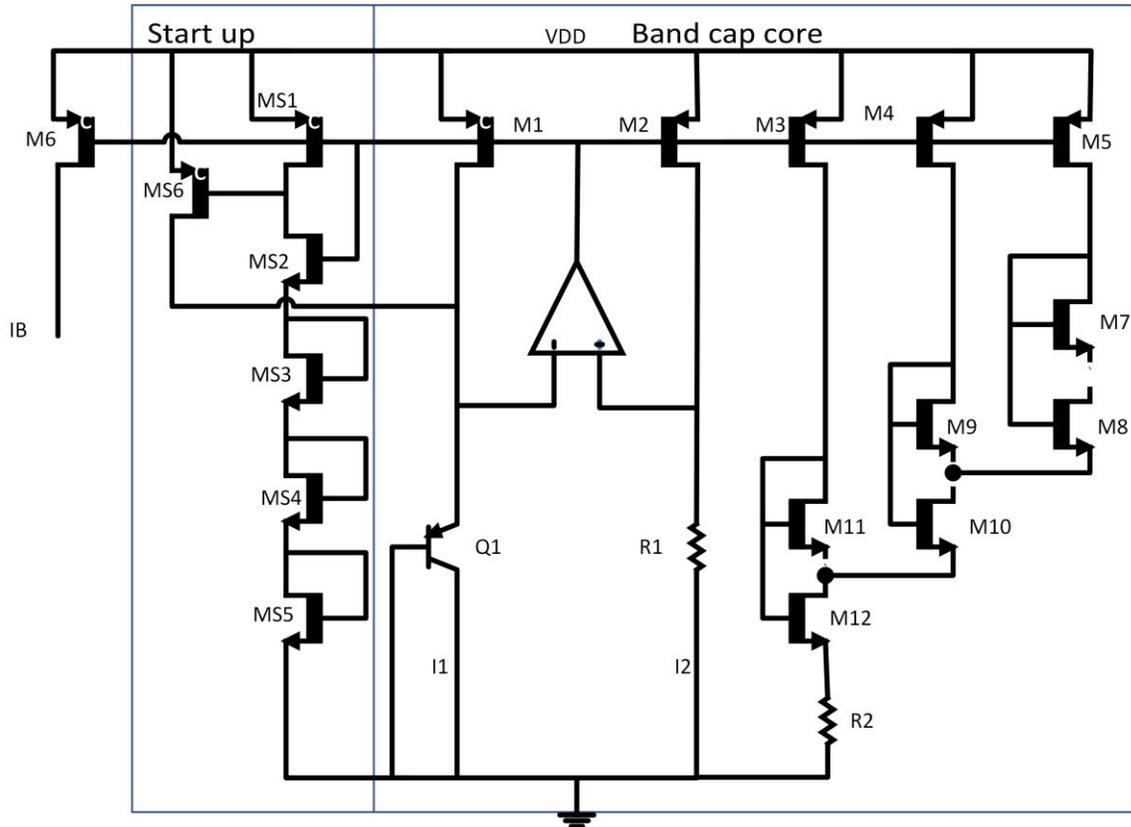
Figure 4-2 Bandgap core
