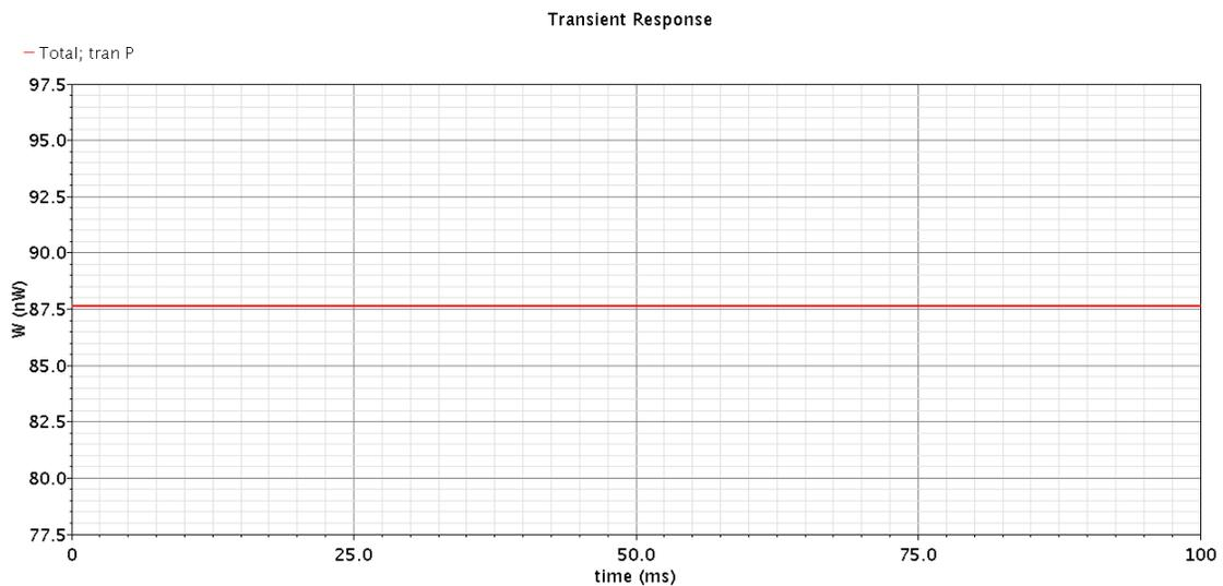
**Figure 4-7 power consumption of the band gap**
