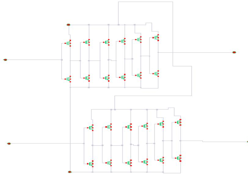
**Figure 5-8 Buffer schematic**
