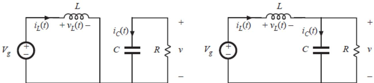
**Figure 2-6 Modes of operation a CCM Boost converter**
