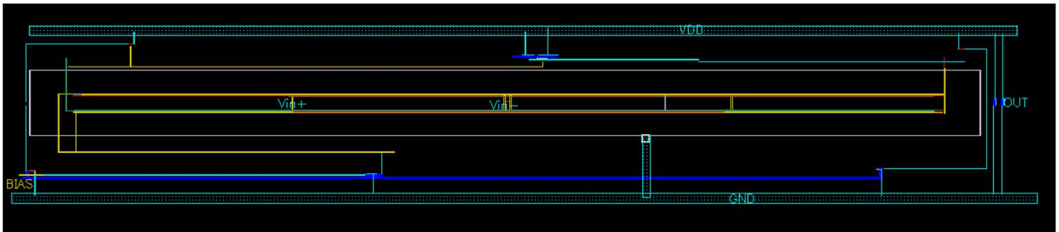
**Figure 2-35 Layout of hysteresis comparator**
