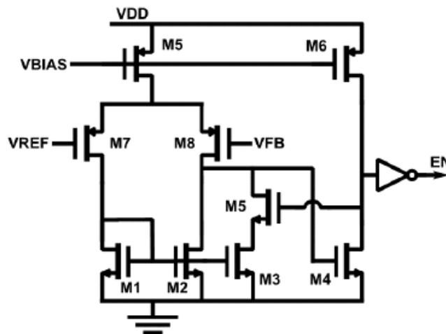
Figure 3-16: Feedback comparator circuit
