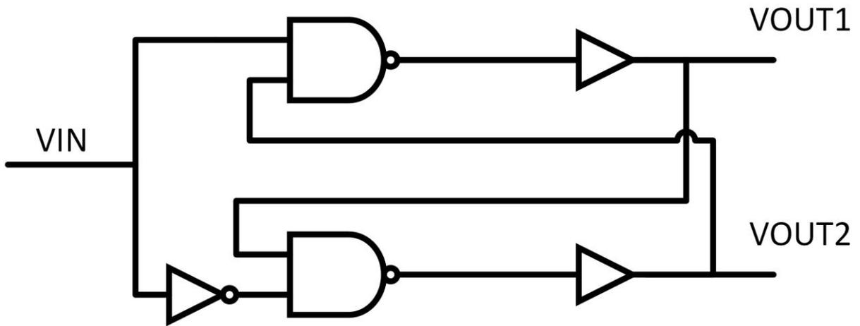
**Figure 5-6 Non-overlapping clock generator schematic**
