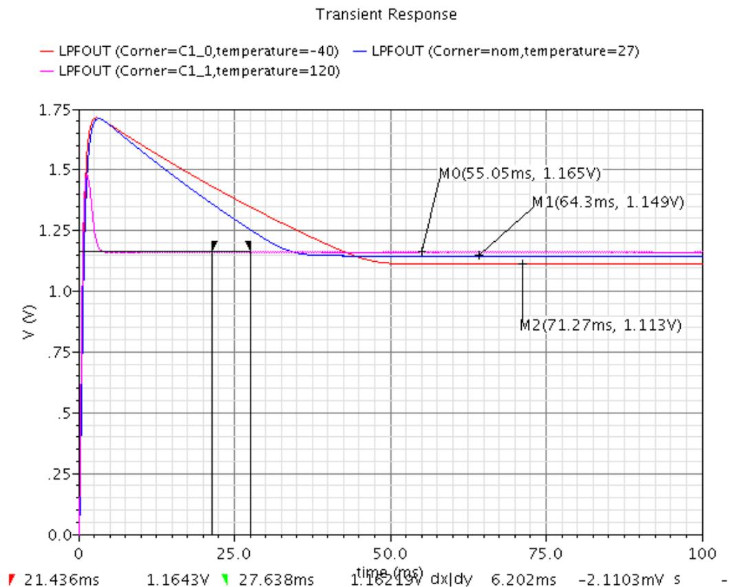
**Figure 2-33 Fast Fast variations of boost converter**
