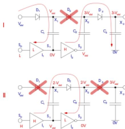
Figure 5-12 two stages of a charge pump
