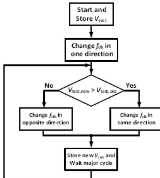
**Figure 2-17 Flow chart of the MPPT loop**
