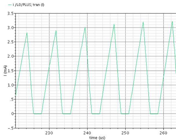
**Figure 2-5 DCM Boost action on current ripples**
