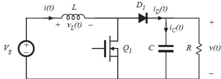
**Figure 2-4 DCM Boost Converter**
