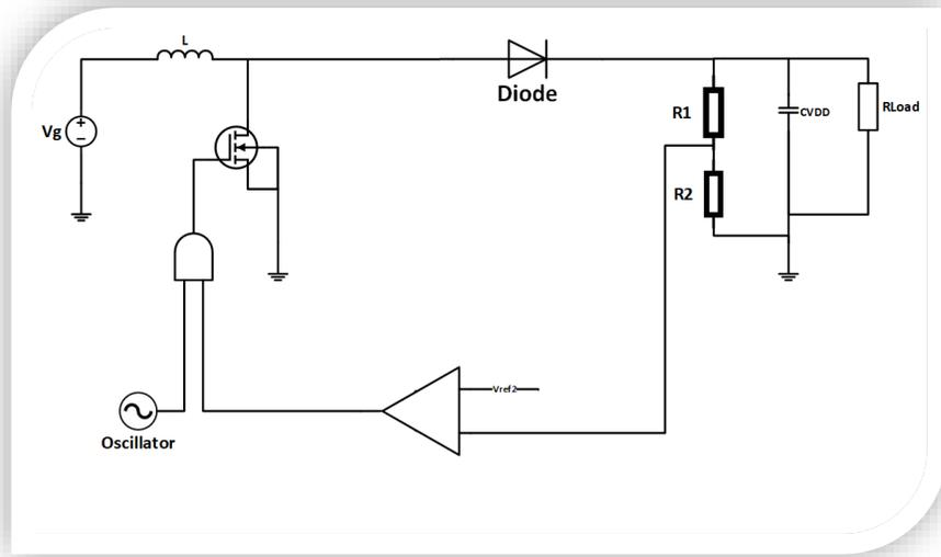
**Figure 3-10: Block diagram of output regulation loop**
