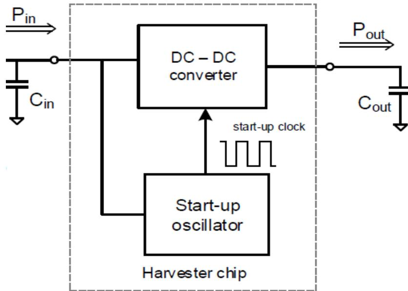
**Figure 5-1 structure of a cold start unit**
