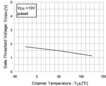
Figure 2: Threshold Temperature Characteristics
