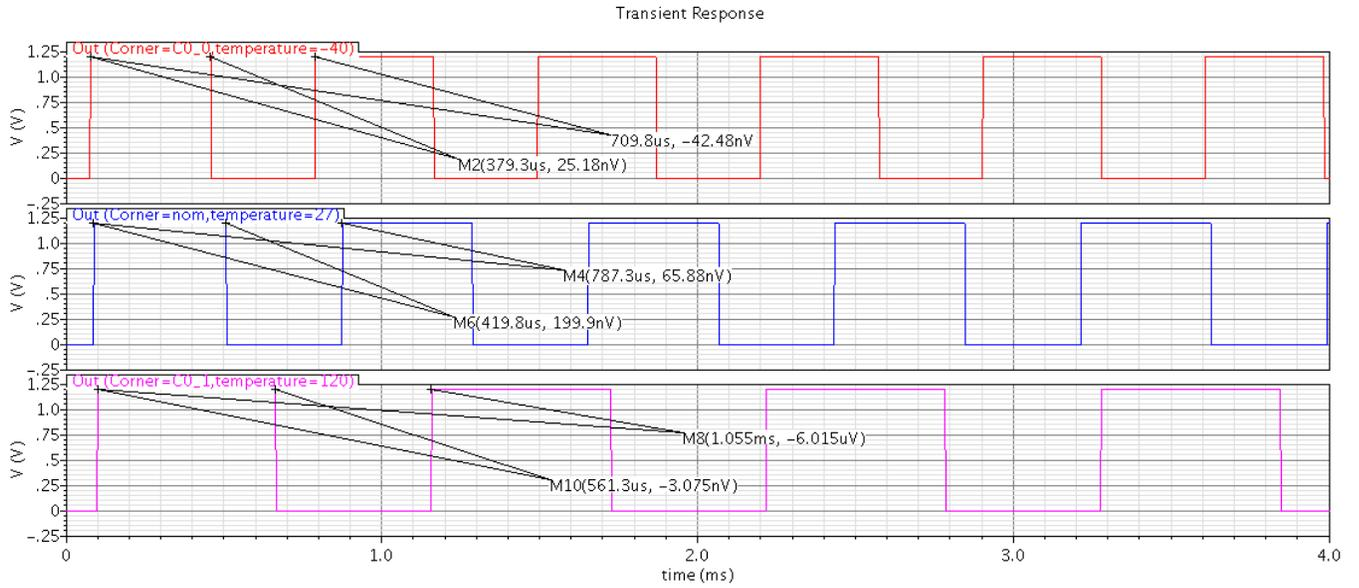
**Figure 2-30 DCO fast fast simulations for -40 and 125°C**
