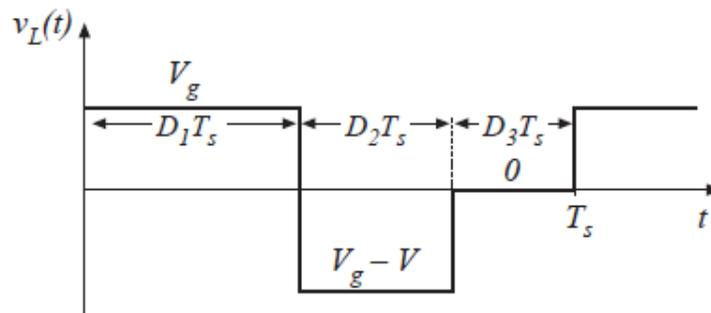
**Figure 2-12 the voltage across time on the inductor**
