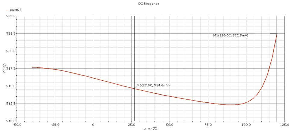
**Figure 4-10 voltage variation with temperature at SS corner**
