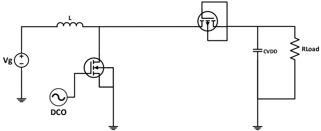
**Figure 2-13 DCM with diode implemented as PMOS**
