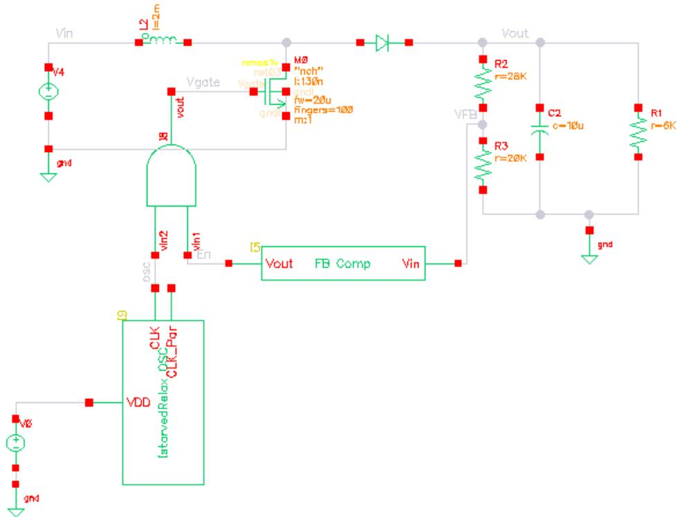
**Figure 3-18: Test bench of output regulation loop**
