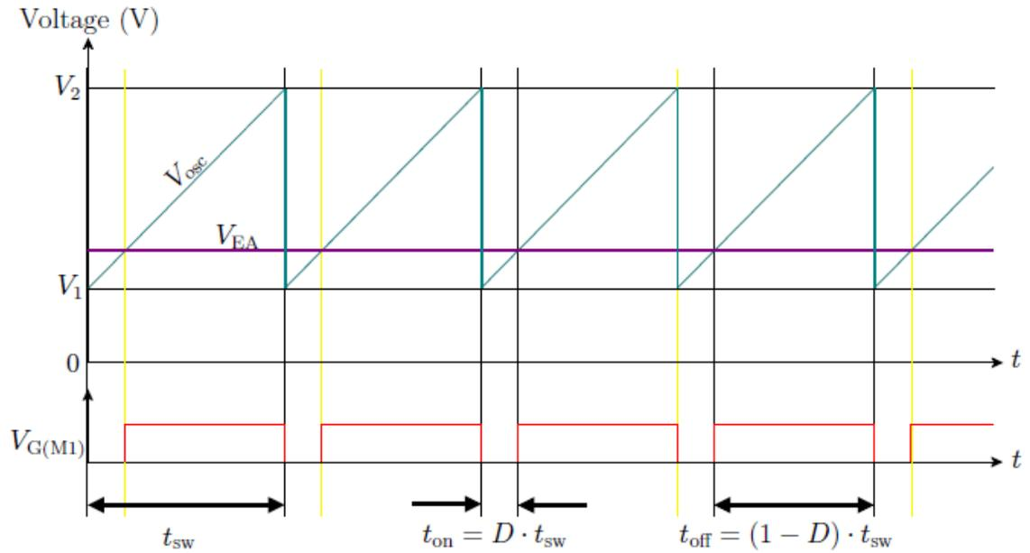
**Figure 3-7: Steady-state timing diagram of a PWM switching converter**
