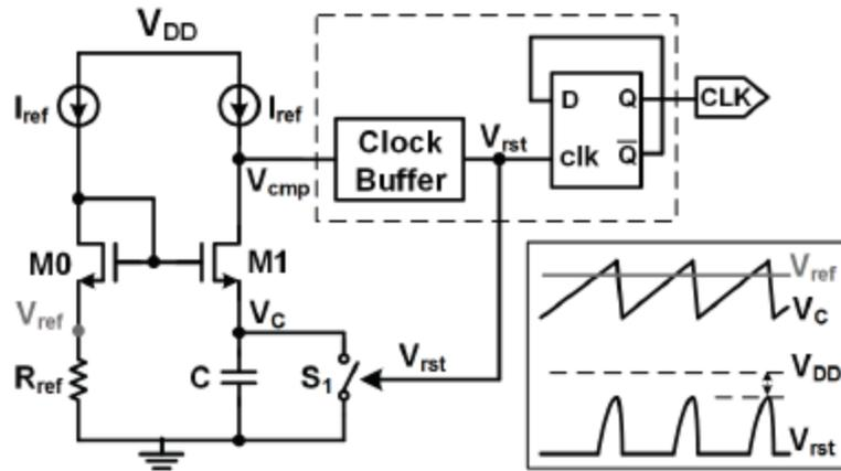
**Figure 3-13: Single-phase current-mode relaxation oscillator and timing diagram**
