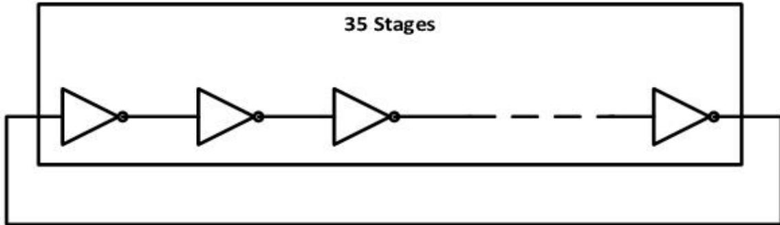
Figure 5-2 Oscillator schematic
