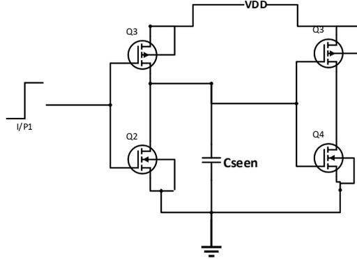
**Figure 2-19 simple two stages of the ring oscillator**
