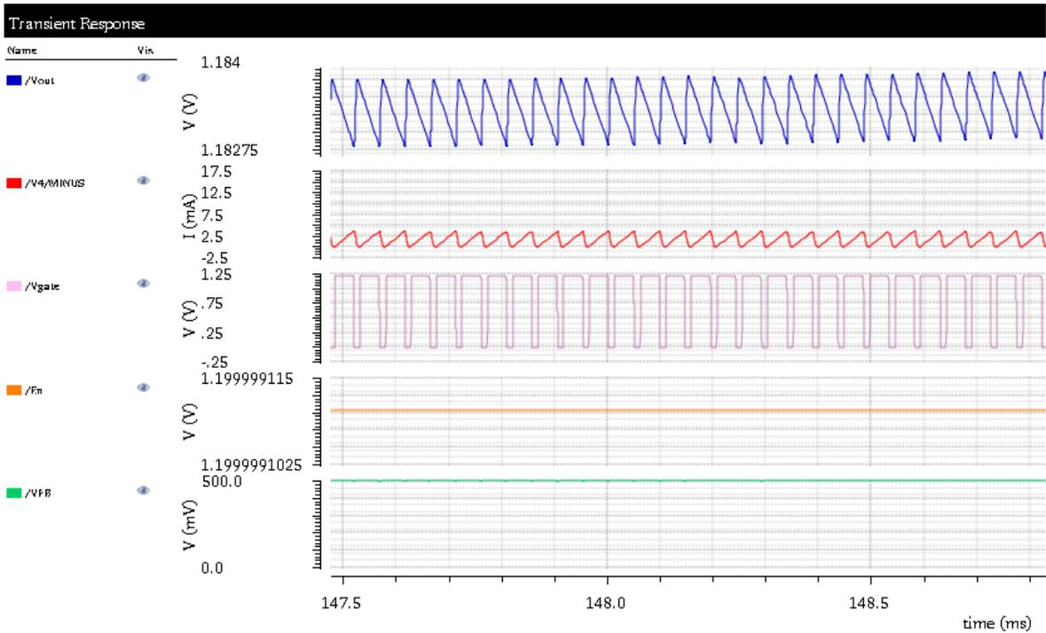
**Figure 3-20: Magnifying the simulation results of the output regulation stage at  $V_{in} = 200$  mV**
