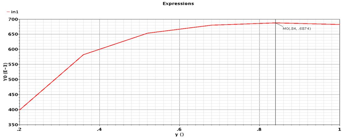
Figure 5-16 charge pump efficiency at different input voltages @Rout= 13M
