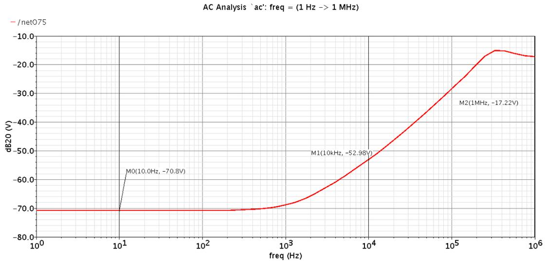
**Figure 4-8 PSRR of the bandgap**
