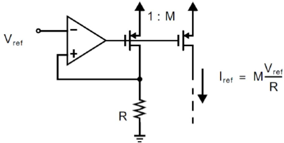
**Figure 4-20** voltage to current converter
