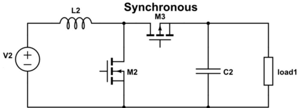
**Figure 3-6: Synchronous Boost Converter**
