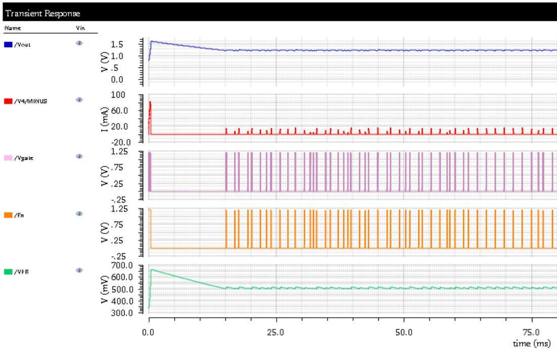
**Figure 3-23: Simulation results of the output regulation stage at  $V_{in} = 900 \text{ mV}$**
