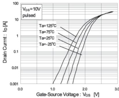
Figure 1:  $I_D$ - $V_{GS}$  Characteristics
