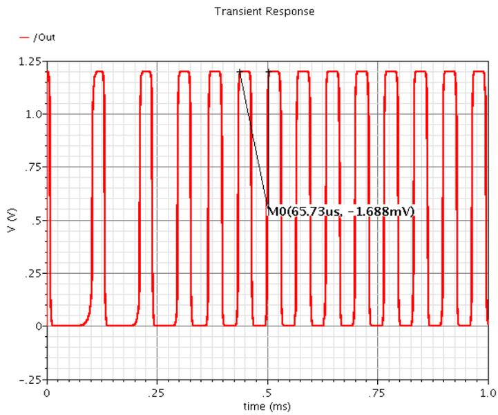
**Figure 2-39 DCO output for 1111 input**
