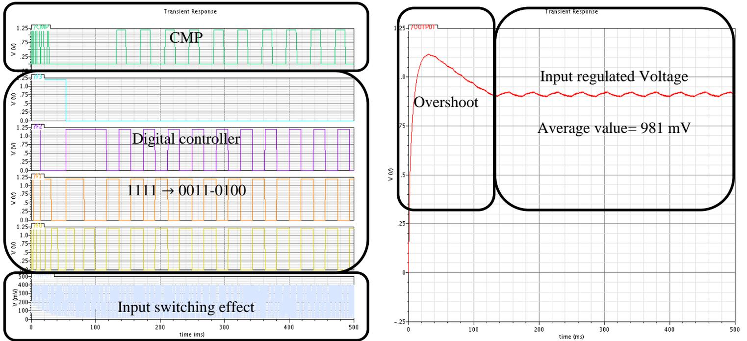
**Figure 2-24 400 mV, 250 Ω test model results**
