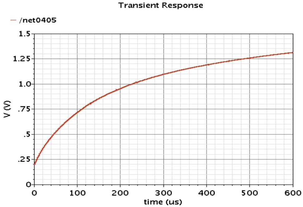
**Figure 5-20 cold star output @ SS corner**
