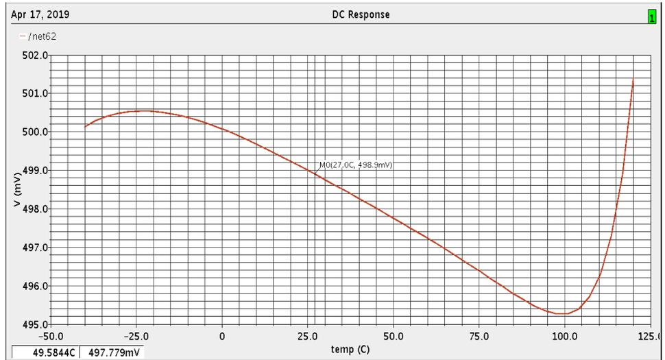
**Figure 4-14 output voltage variations at FF corner after using a trimming circuit**
