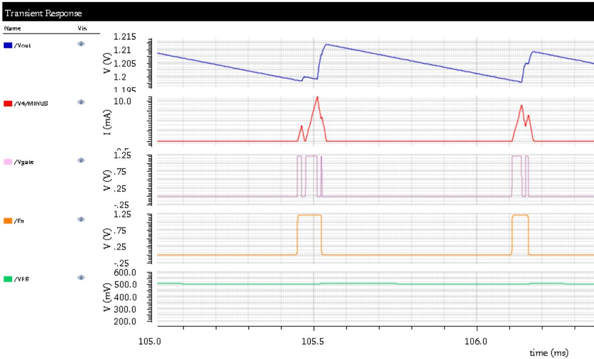
**Figure 3-22: Magnifying the simulation results of the output regulation stage at  $V_{in} = 600 \text{ mV}$**
