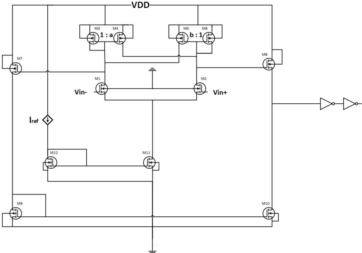
**Figure 2-15 Hysteresis comparator using current unbalance**
