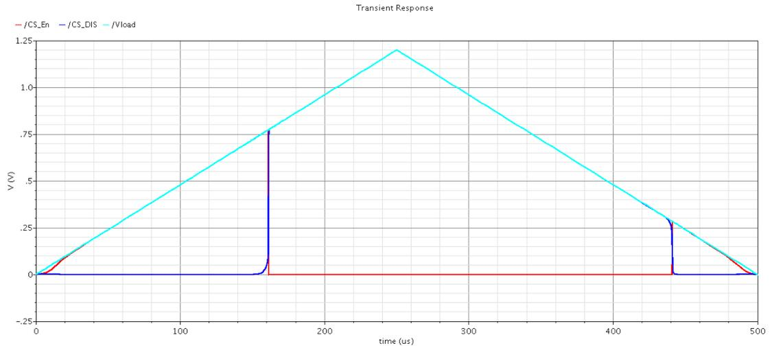
**Figure 2: Transient response of cold start comparator while increasing and decreasing its VDD**
