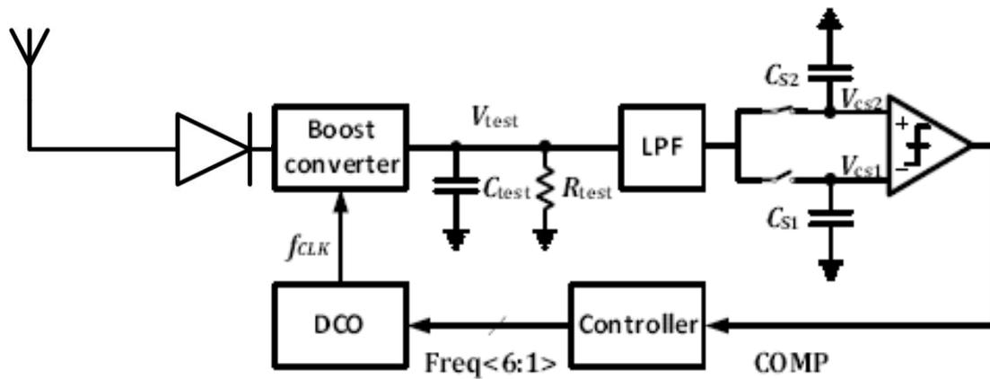
**Figure 2-2 Block Diagram of MPPT**
