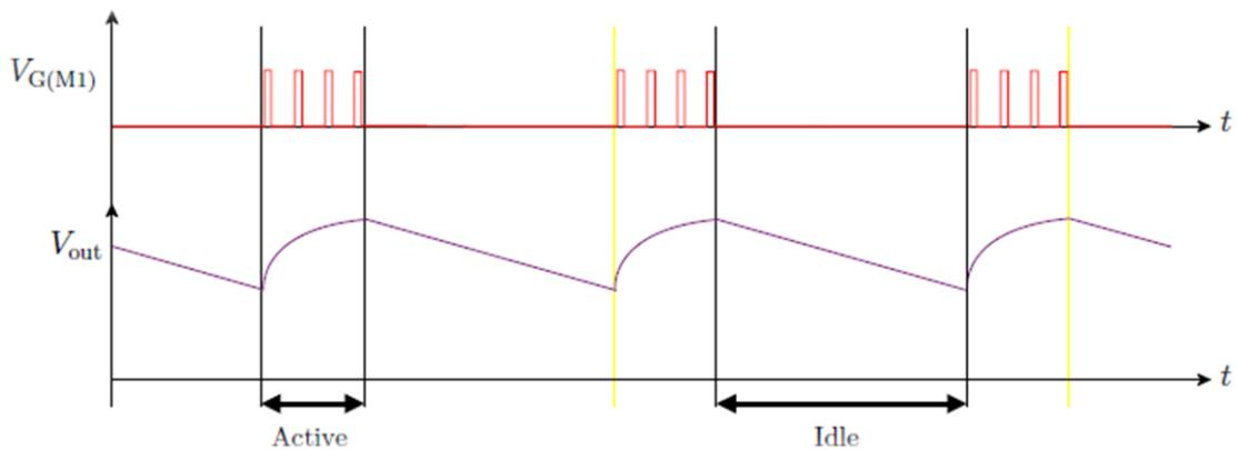
**Figure 3-8: Signal waveforms of the PFM operation control in steady-state.**
