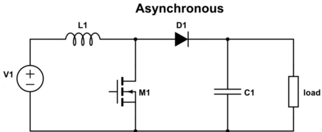
**Figure 3-5: Asynchronous Boost Converter**
