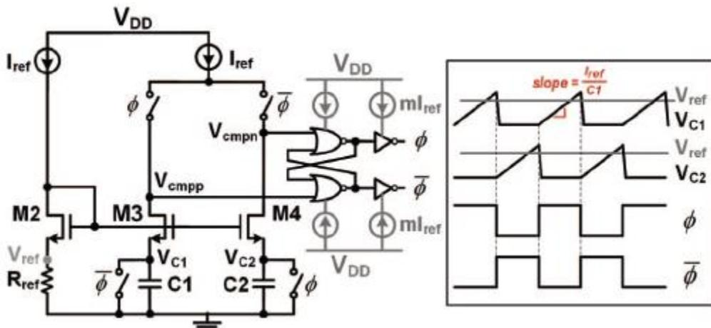
Figure 3-14: dual-phase current-mode relaxation oscillator and its timing diagram
