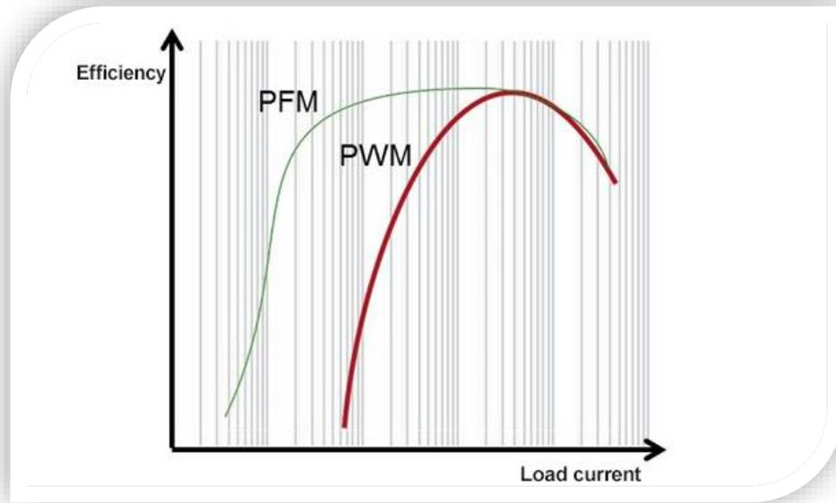
**Figure 3-9: Efficiency characteristics of PWM and PFM illustrated**
