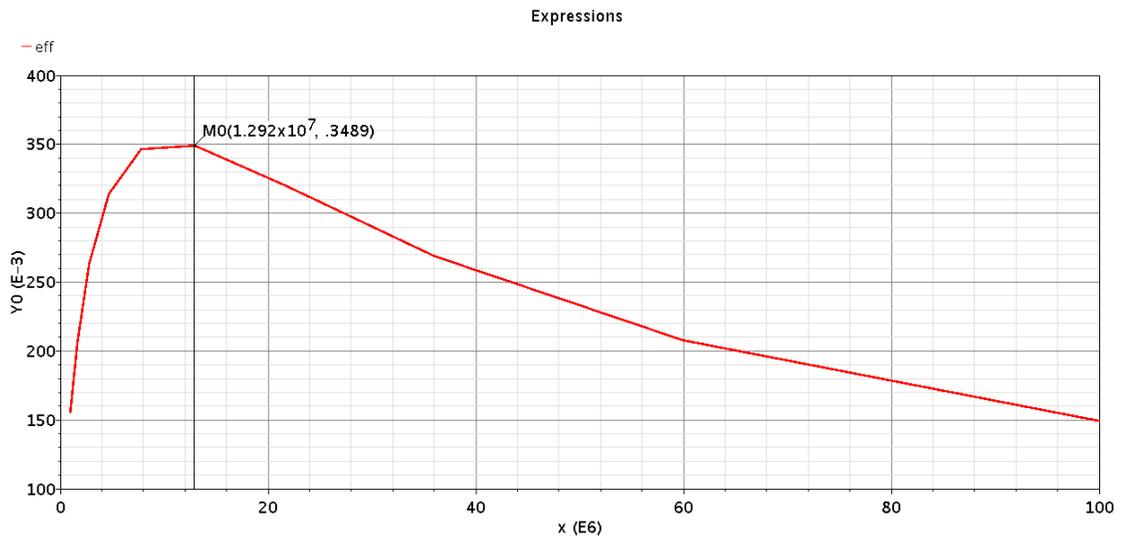
**Figure 5-15 charge pump efficiency at various loads**
