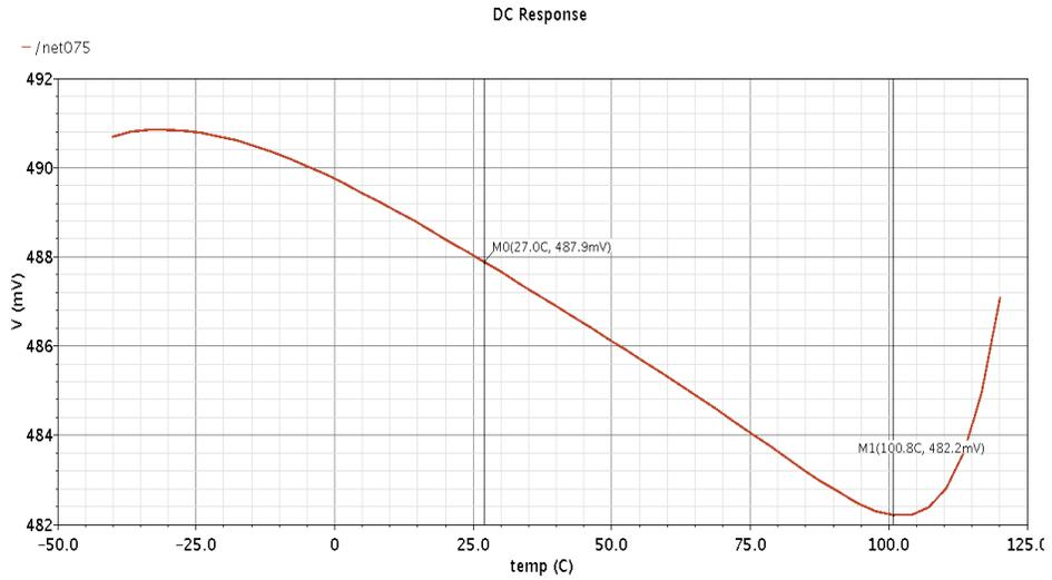
**Figure 4-11 voltage variation with temperature at FF corner**
