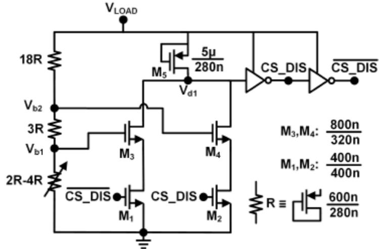
**Figure 1: Cold start comparator with hysteresis**
