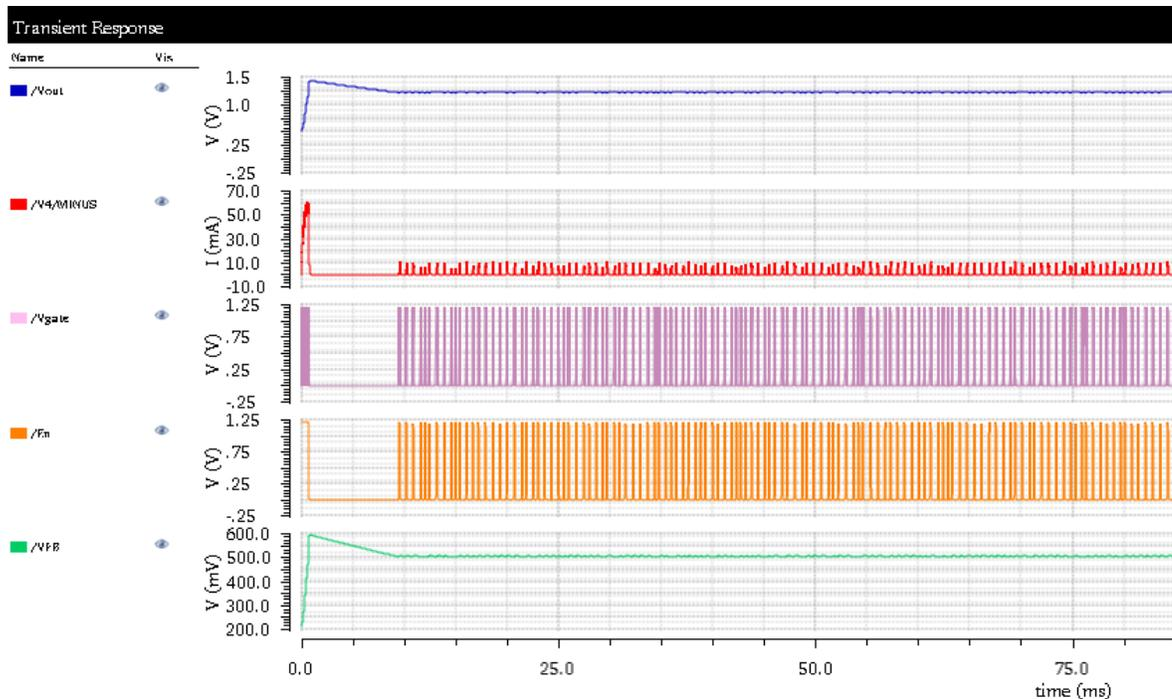
**Figure 3-21: Simulation results of the output regulation stage at  $V_{in} = 600 \text{ mV}$**
