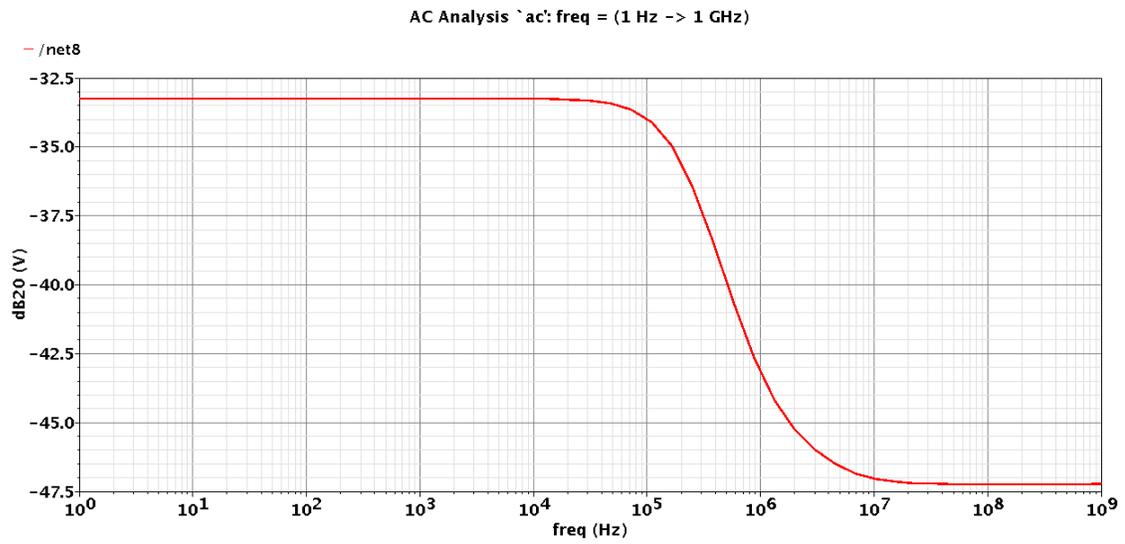
Figure 4-16 op-amp simulation DC gain
