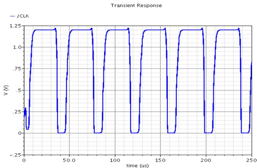
**Figure 3-15: Transient response of the designed oscillator**
