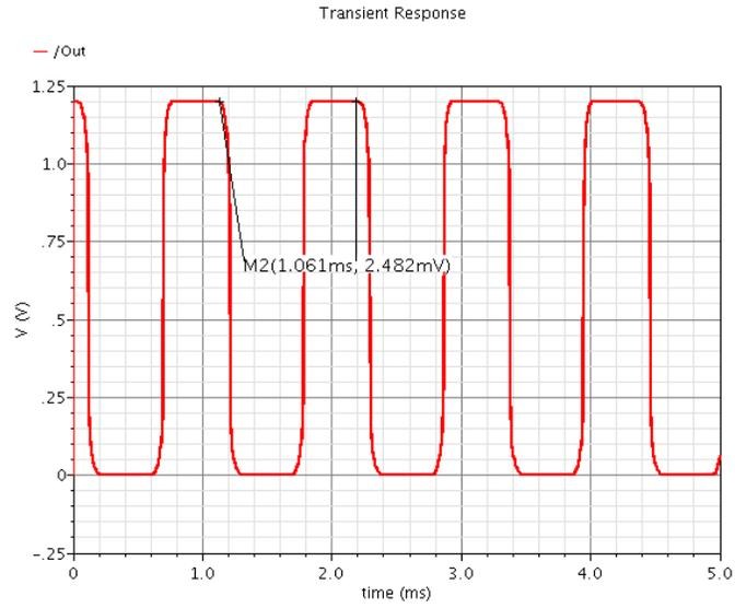
**Figure 2-38 Post-layout result for DCO output for 0000 digital input**
