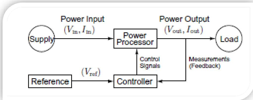
**Figure 3-1: Block diagram of a typical electronic power conversion system.**
