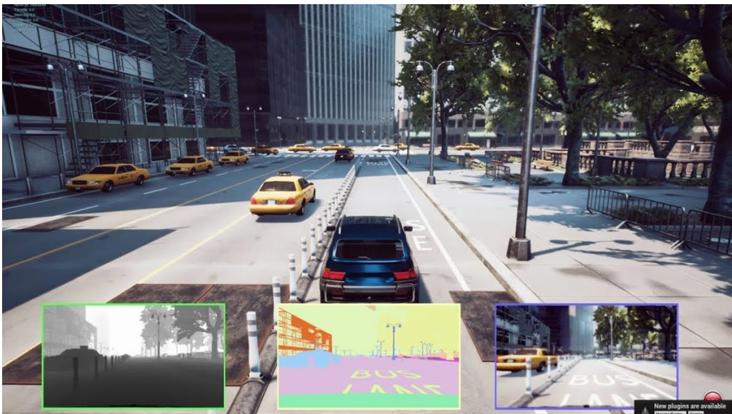
Figure 11. A screen capture of a scene taken from AirSim, showing several live sensor data it has to offer.
