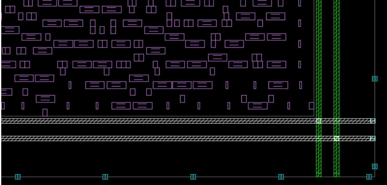
Figure 115: Zoomed in view of power rings and floorplanning placement
