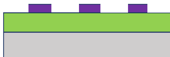
D- Develop the photo-resist using the mask of the IDTs and reflectors (Leaving their pattern uncovered)
