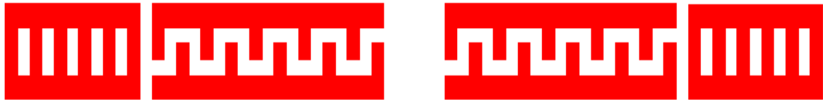
Figure 99-Five Pairs two-ports SAW MEMS resonator fabrication mask
