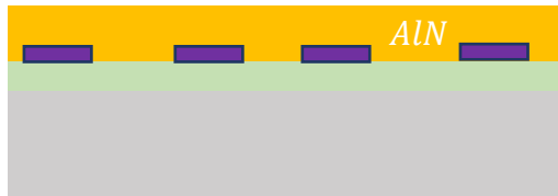
C- Deposit AlN to act as the piezoelectric material (Sputtering preferred)
