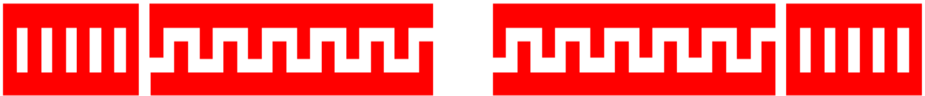
Figure 96-Six Pairs two-ports SAW MEMS resonator fabrication mask
