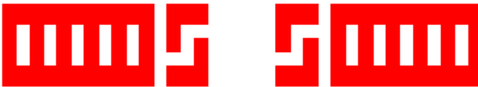
Figure 93-One Pair two-ports SAW MEMS resonator fabrication mask
