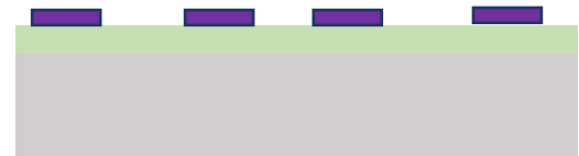
B- After performing the RIE to SiO_2
