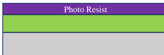
C- Spin-coat photo resist
