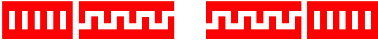
Figure 98-Four Pairs two-ports SAW MEMS resonator fabrication mask
