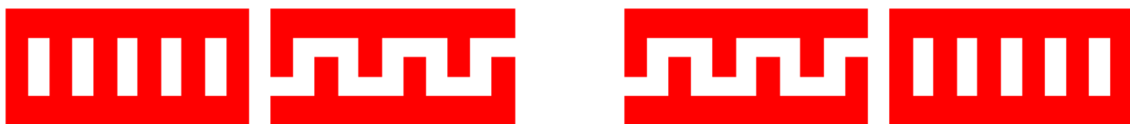
Figure 95-Three Pairs two-ports SAW MEMS resonator fabrication mask
