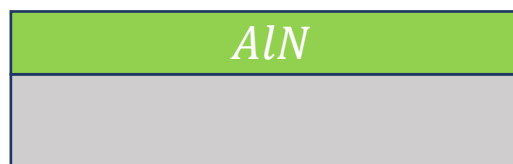
B- Deposit AlN to act as the piezoelectric material
