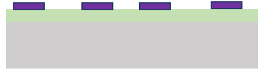
B- After performing the RIE to SiO_2
