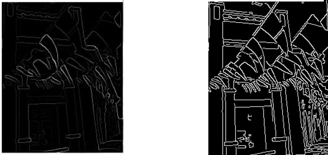
Figure 12: Step 3: Non-maximum suppression, step 4: Hysteresis thresholding
