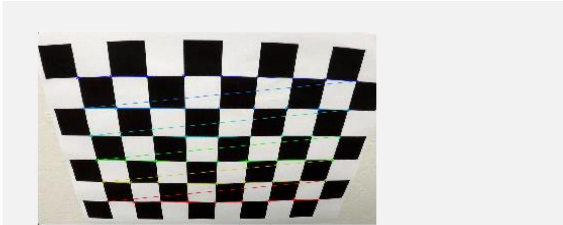
Figure 5: chessboard corners traced on a sample image
