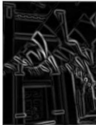
Figure 11: step1: After grayscale and gaussian filter, step 2: compute magnitude and angle
