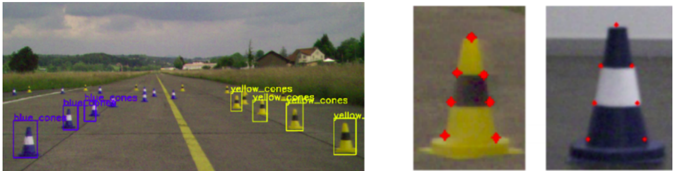
Figure 4.12: Cone batches (left) and Cone batches with key points detected (right)
