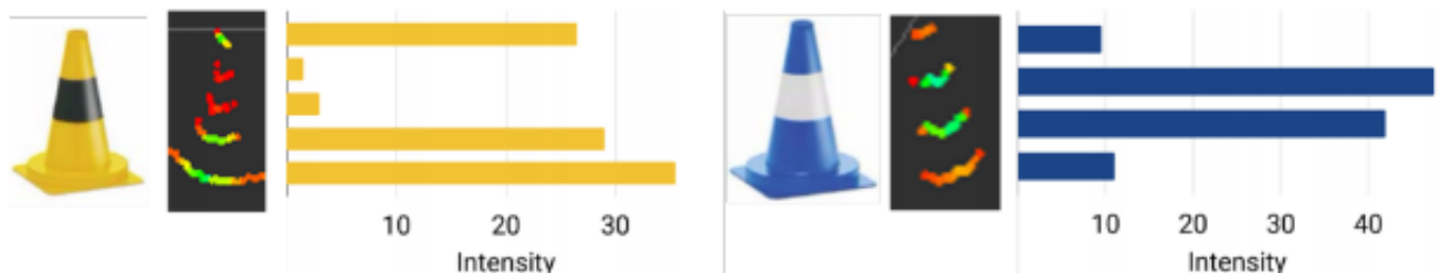
Figure 3.5: The intensity gradients for the pre-defined yellow and blue cones along with their point cloud returns.
