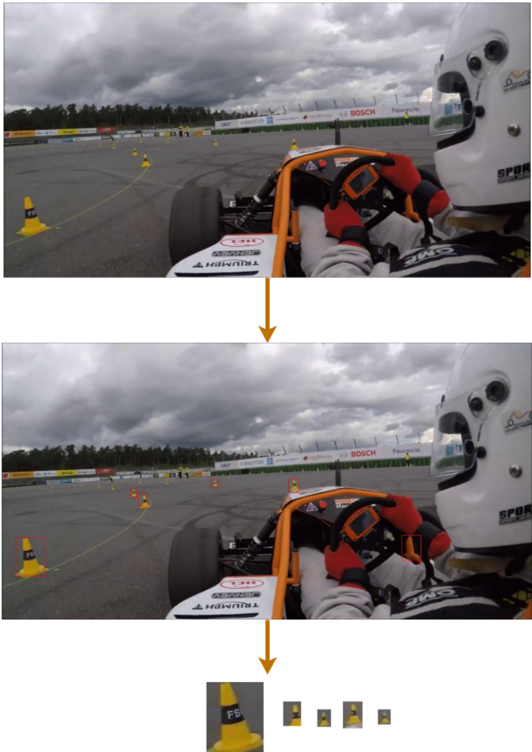
Figure 5.6: Testing the detection module in cloudy climate condition
