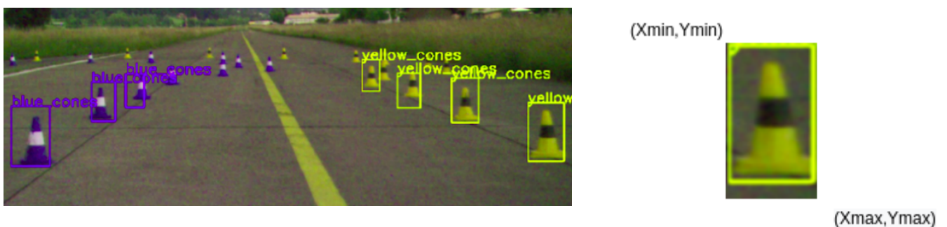
Figure 4.20: 2D Cone bounding box detection(left) boundary box points (right)
