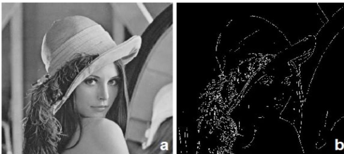
Figure 11: (a) Original Image, (b) Sobel Operator Output.
