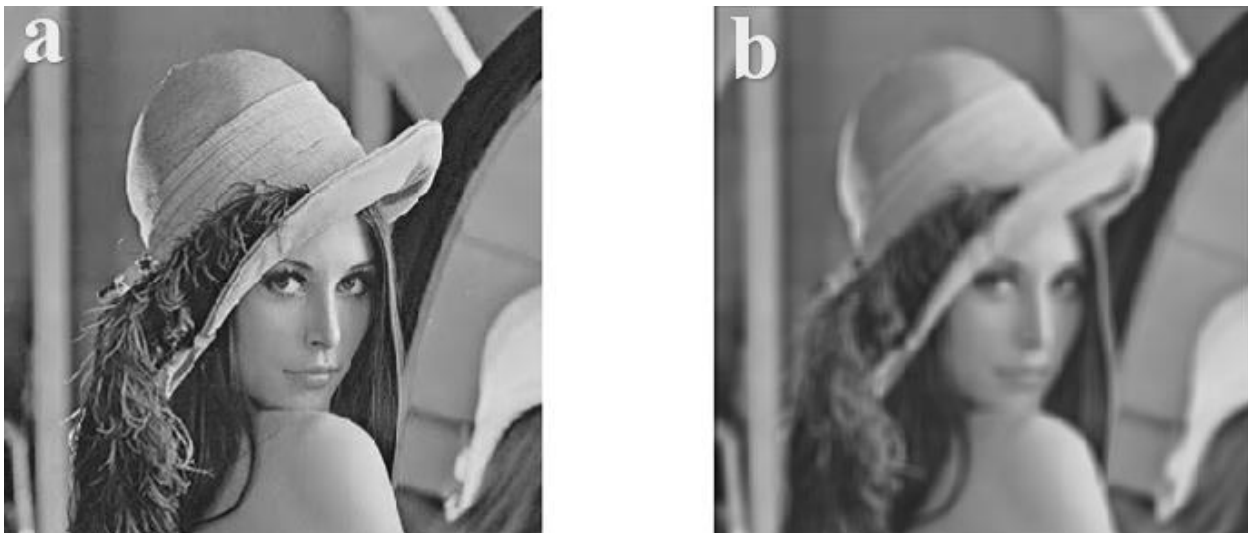
Figure 13: (a) Original Image, (b) Gauss Operator Output.
