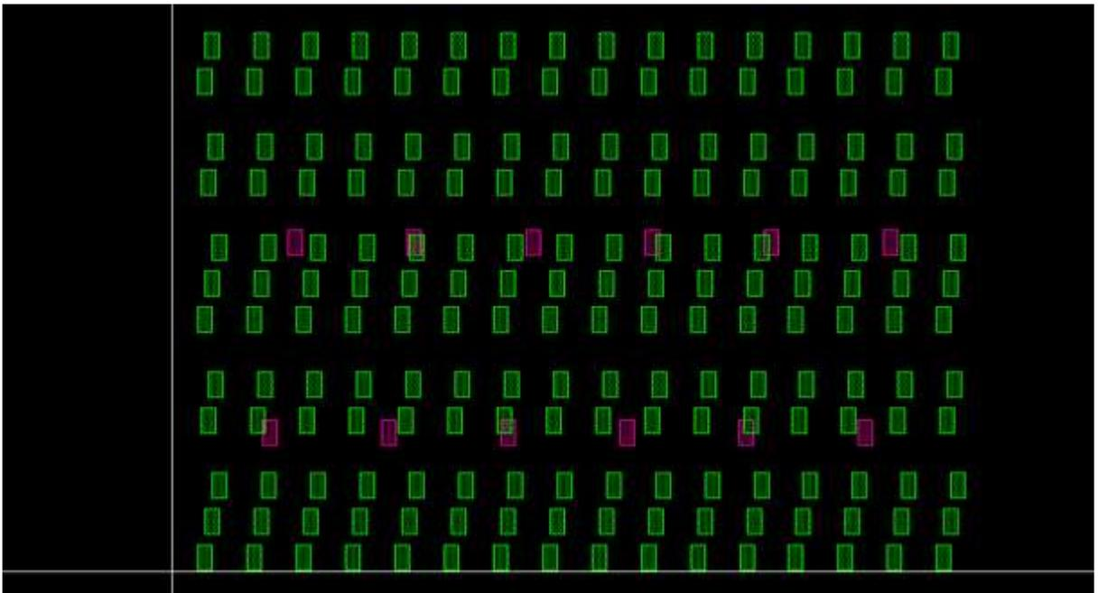
*Figure 4.3.2 (k) the filling cell layout*
