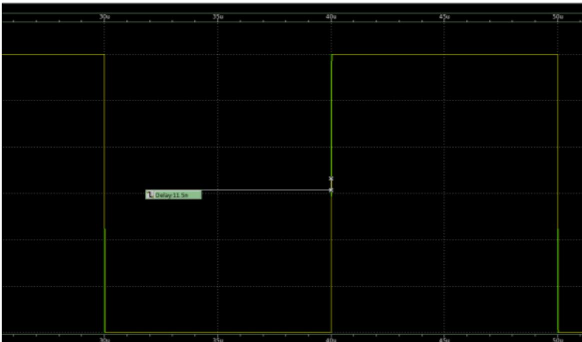
Figure 3.4.3 (c): Delay of two inverters connected with a very long interconnect
