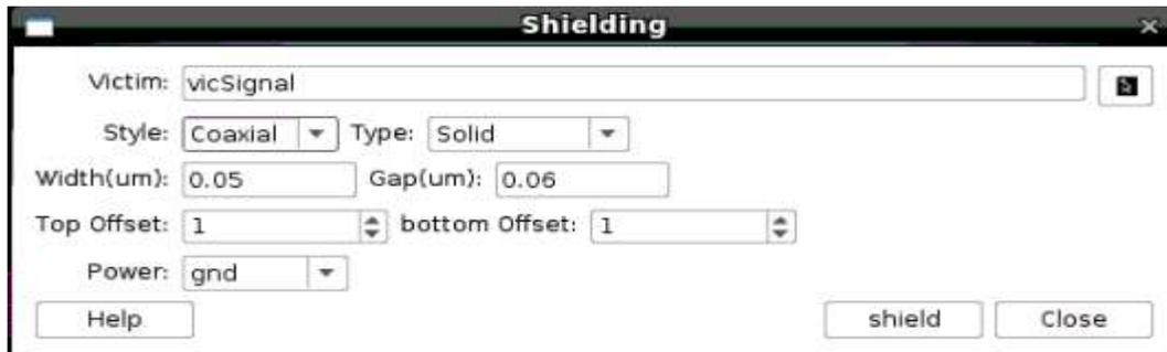
Figure 3.6.7(a) Shielding tool GUI
