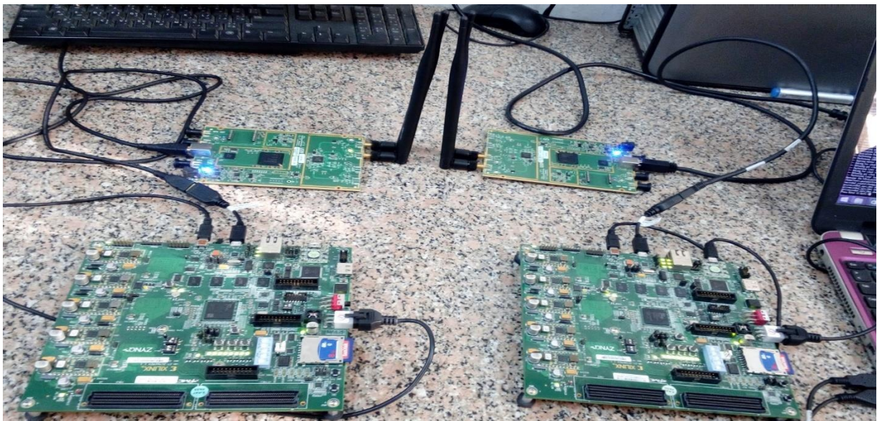
Figure 7-1 Transmitter and Receiver hardware full chain
