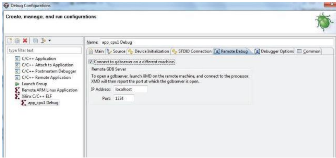
Figure 6-8 CPU1 remote debug configuration
