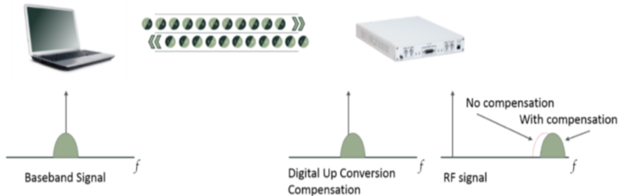
Figure 3-2 Center Frequency fine tuning
