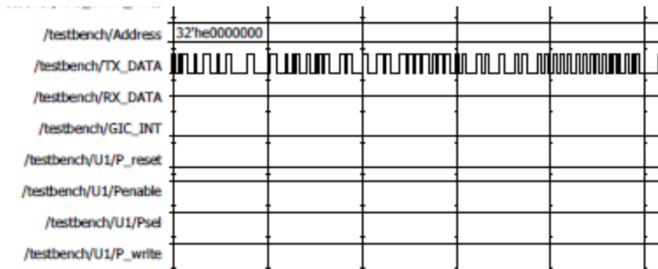
Figure 4-7 interrupt is raised and the data is totally sent
