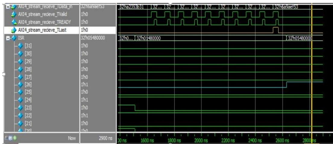
Figure 6-14 RC bit 26 goes high after TLAST
