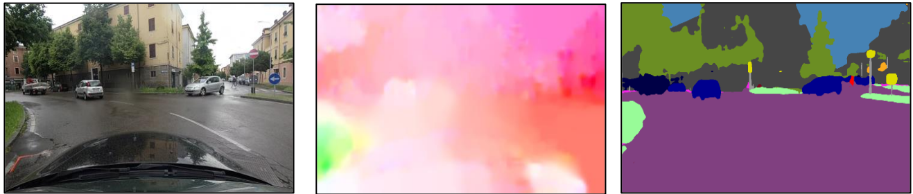
Figure 4 From the left : Main frame from roof mounted camera , Optical flow of the scene & Semantic segmentation of the scene
