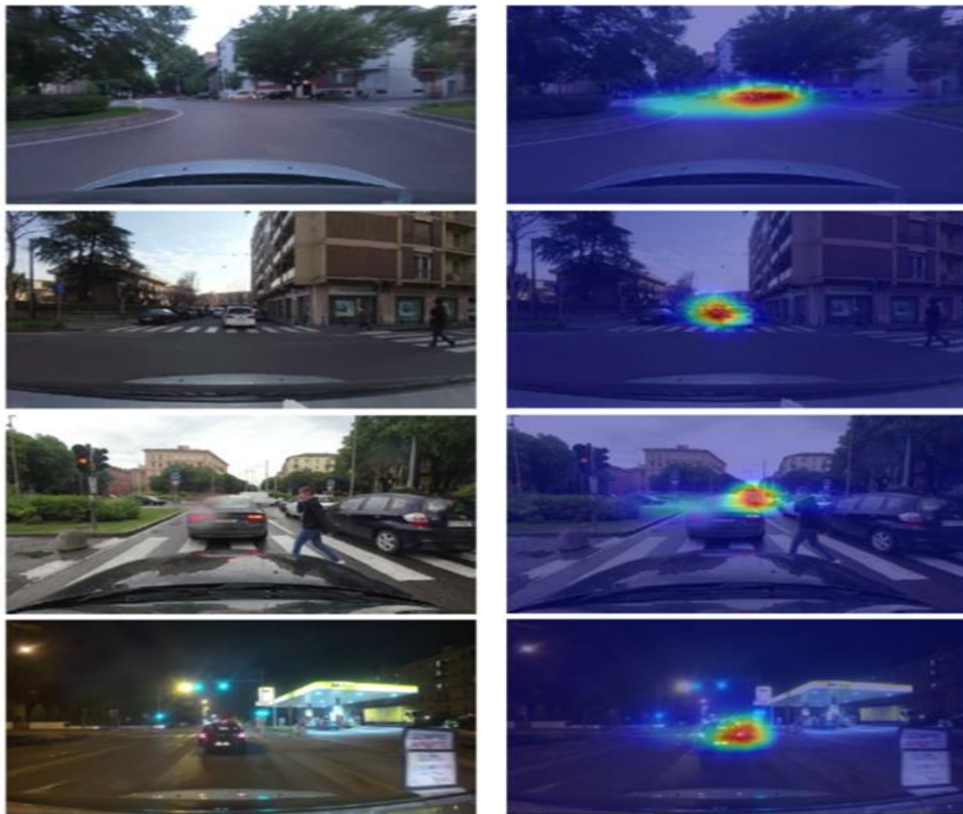
Figure 7 from the left : Main frame & gaze map output of the Gaze Network overlaid on the main frame.
