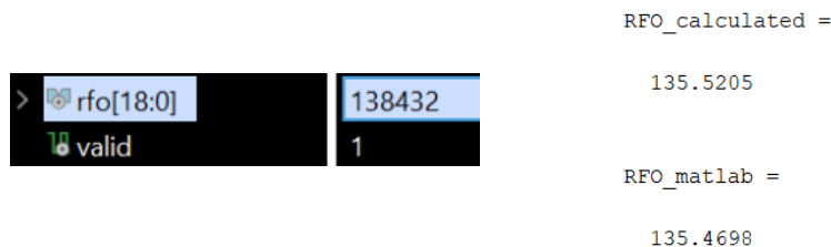
Figure [79]: Fine Synchronizer RTL Results
