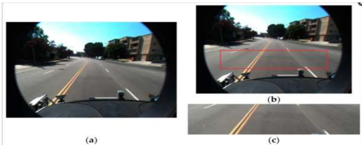
Figure 39: (a) Input image of the camera (b) Apply fixed ROI on the input (c) The Output
