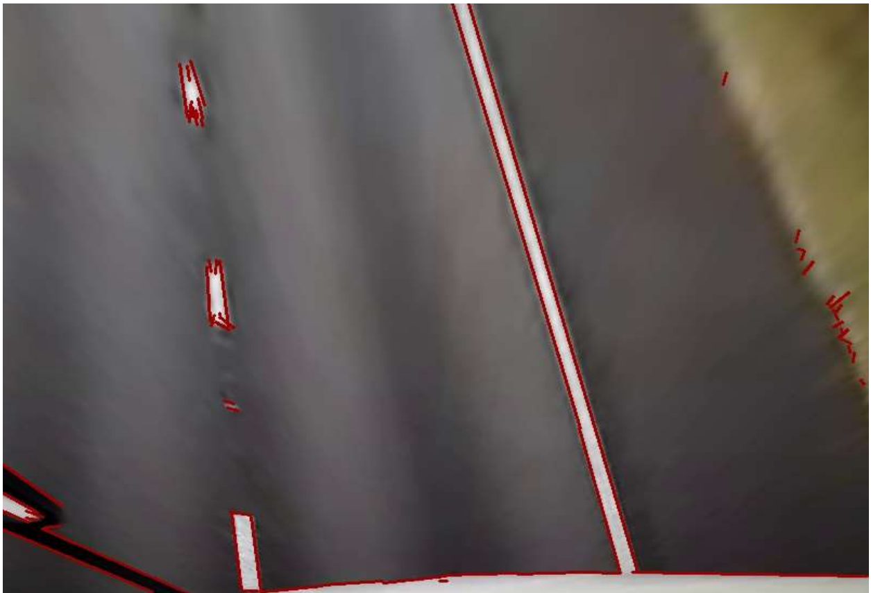
Figure 50: LSD before filtration
