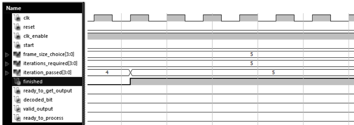
Figure 6-13: handshaking signals: Finished
