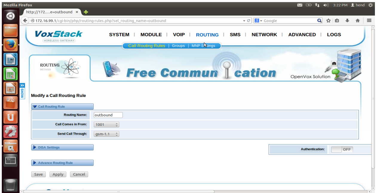
Figure 8-8 set up Routing Rule (outbound)
