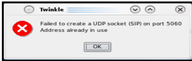
Figure 8-10 : error after installation
