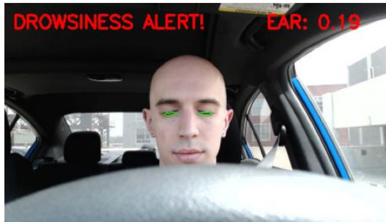
Figure 14: Sound an alarm if the eyes have been closed for a sufficiently long enough time
