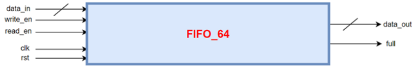
Figure 54: Block diagram of module of FIFO_64
