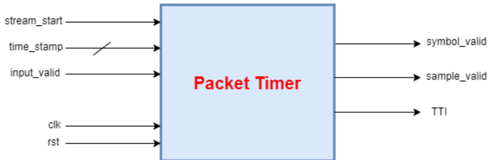
Figure 76: Block diagram of module packet_timer
